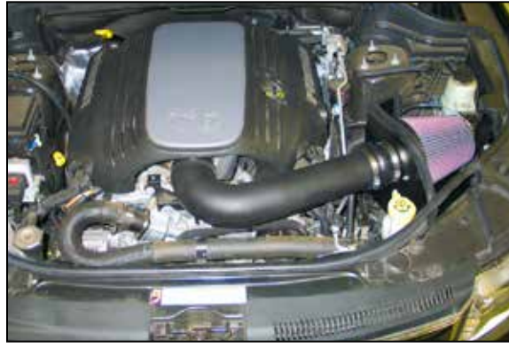
29. Reconnect the vehicle's negative battery cable. Double check to make sure everything is tight and properly positioned before starting the vehicle.
