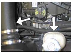
23. Install the provided silicone hose onto the factory crank case vent tube and then connect the open end to the 90° fitting installed into the K&N® intake tube.
