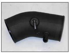
17. Install the provided 90° vent fitting into the  $K\&N^{\otimes}$  intake tube as shown.
