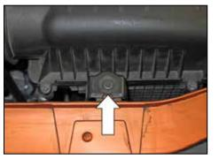
6. Remove the bolt that secures the air box to the core support.
