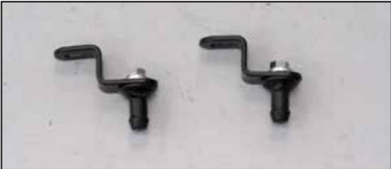
11. Install the two provided mounting studs onto the two heat shield brackets (070061) as shown.
