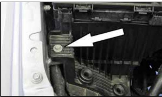
9. Remove the bolt shown that secures the air box mount bracket to the inner fender.
