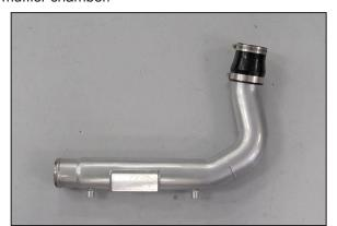
11. Install the provided step coupler (5-255) onto the K&N® intercooler pipe and secure with the provided hose clamp.
