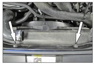
10. Install the two provided rubber mounted studs into the core support as shown. The studs will thread into the holes for the bolts which secure the muffler chamber.
