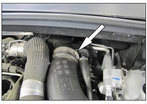
Loosen the hose clamp securing the intake tube to the turbo inlet pipe.
