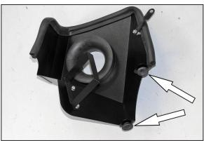
19. Install the air filter housing grommets into the heat shield as shown.
