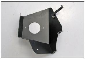
14b. On 2016 and later model vehicles, install bracket (064343) onto the heat shield as shown using the provided hardware and spacer.
