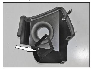
17. Install the fresh air intake scoop mounting bracket onto the heat shield and secure with the provided hardware.
