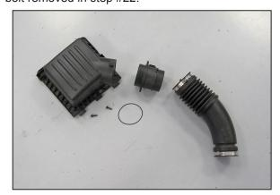
24. Remove the mass air sensor from the upper air filter housing and disconnect the intake tube. NOTE: Remove the O-ring from the mass air sensor housing.
