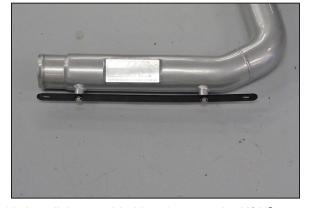
12. Install the provided bracket onto the K&N<sup>®</sup> intercooler pipe and secure with the provided hardware.
