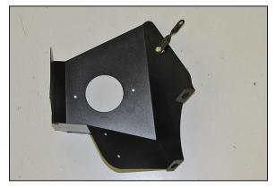
14a. On 2015 and earlier model vehicles, install bracket (070702) onto the heat shield as shown using the provided hardware and spacer.
