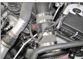
28. Reconnect the mass air sensor electrical connection and install the wiring harness retaining clip into the flange on the mass air sensor as
