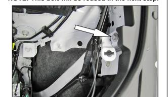
22b. On 2016 and later model vehicles, remove the fender mounting bolt shown.
