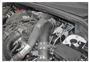
27. Install the provided coupling hose (08186) onto the mass air sensor housing, and then install the K&N® intake tube into the hose. Install the tube and mass air sensor assembly onto the filter adapter and into the coupler at the turbo inlet. Adjust the mass air sensor and intake tube for best fit and then secure with the provided hose clamps. NOTE: once everything is adjusted, secure all six of the hose clamps.
