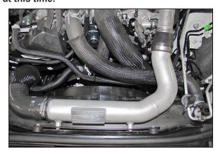
13. Install the intercooler pipe assembly and secure with the provided hose clamps and hardware, tighten the bracket mounting bolts at this time.
