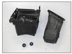
18. Remove the fresh air intake scoop and two of the mounting grommets from the lower air filter housing.
