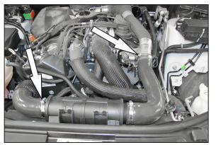
8. Loosen the inter cooler hose to pipe and hose to muffler chamber hose clamps,
