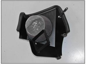
20. Install the K&N® air filter onto the filter adapter and secure with the provided hose clamp.
