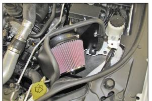
23. Install the heat shield assembly onto the air filter mounting studs and place the mounting bracket in position and the secure with the factory bolt removed in step #22
