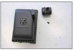
9. Remove the mass air sensor from the factory upper air filter housing.
