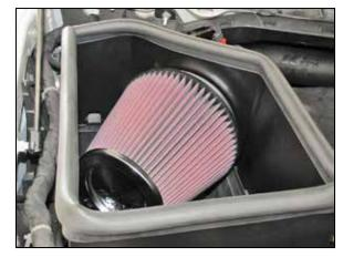
16. Install the K&N<sup>®</sup> air filter onto the filter adapter and secure with the provided hose clamp. NOTE: Drycharger<sup>®</sup> air filter wrap; part # RF-1042DK is available to purchase separately. To learn more about Drycharger<sup>®</sup> filter wraps or look up color availability please visit http://www.knfilters.com<sup>®</sup>.
