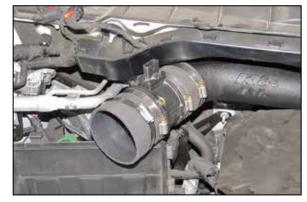
11. Install the mass air sensor into the coupling hose installed onto the  $K\&N^{\otimes}$  intake tube.
