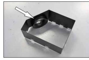
12. Install the provided radius adapter into the heat shield and secure with the provided hardware.
