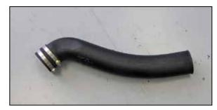
7. Install the provided coupling hose (08690) halfway onto the K&N<sup>®</sup> intake tube and secure with the provided hose clamp as shown.
