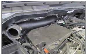
2. Disconnect the mass air sensor electrical connection.
