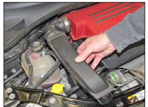
5. Remove the plastic intake tube and coupler as shown.
