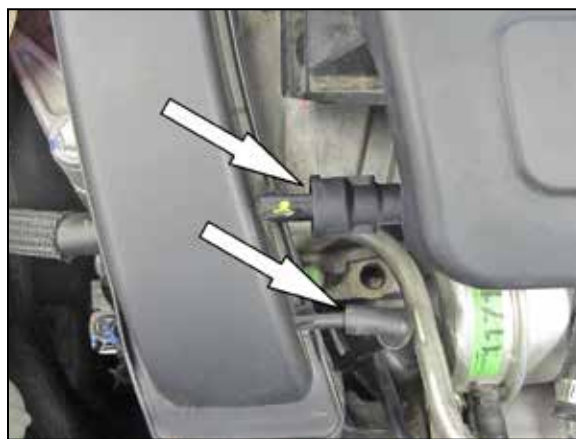
3. Disconnect the vacuum line and crank case vent hose from the plastic intake tube.
