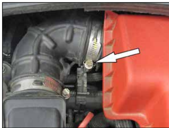
4. Loosen the hose clamp securing the intake hose to the air filter housing.
