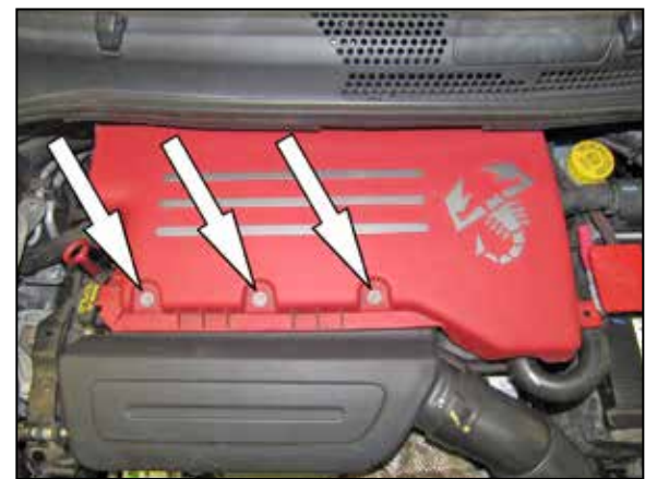
6. Loosen the three screws and remove the air filter housing lid and air filter.
