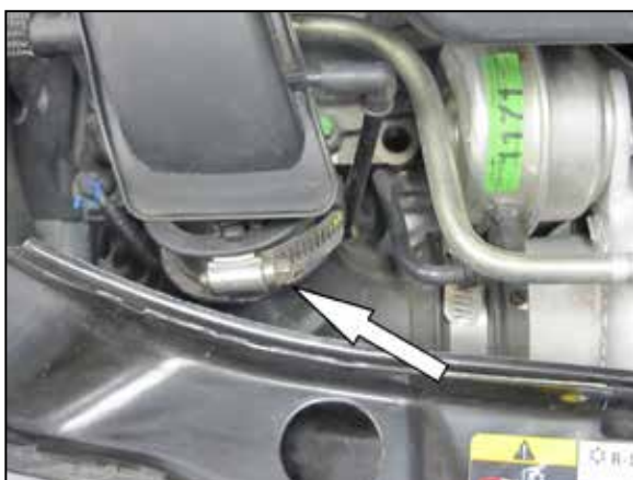
2. Loosen the hose clamp securing the turbo inlet hose to the plastic intake tube.
