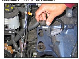
6. Remove the two air box mounting grommets from the bracket as shown.
