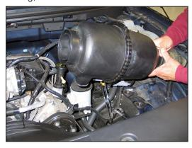
4. Firmly pull up the assembly to unhook it from the mounting grommets and inner fender as shown.
