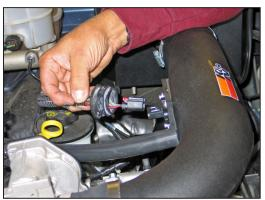
28. Reconnect the mass air sensor secondary connection and then reconnect the remaining end to the mass air sensor.
