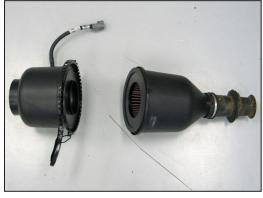
15. Release the clam shell clamp to open the air cleaner assembly as shown.
