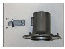
18. Using the supplied T20 TORX, remove the two screws that secure the mass air sensor and then remove the mass air sensor as shown.
