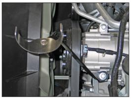
9. Install the tube mounting bracket assembly onto the A/C compressor using the bolt removed in the previous step.
