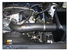
23. Install the intake tube into the silicone hose at the throttle body and align with the saddle clamp. Secure the intake tube with the provided hose clamp.
