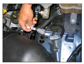
5. Unhook the secondary mass air sensor connection from the clip that secures it to the air box mounting bracket, then disconnect the secondary mass air connection.
