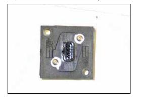
12. Install the mass air sensor onto the mass air sensor adapter with the provided hardware as shown.
