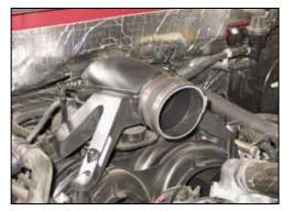
9. Install silicone hose (#08630) onto the throttle body inlet tube with the provided hose clamps as shown.
