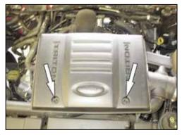
3. Remove the two bolts that secure the engine cover.
