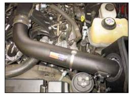
24. Install the intake tube into the air filter assembly and silicone hose at the engine inlet tube, then align with the tube bracket and secure with the provided hose clamps as shown.
