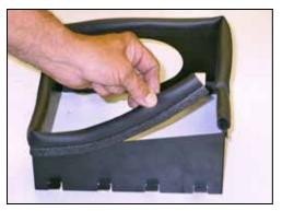
15. Install the long edge trim onto the heat shield as shown.
