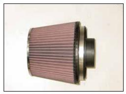
21. Install the air filter adapter into the K&N<sup>®</sup> air filter and secure with the provided hose clamp as shown.
