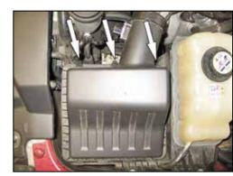
7. Un-snap the three latches securing the upper air box housing to the lower air box housing as shown.
