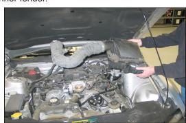
6. Remove the air box assembly from the vehicle. NOTE: K&N Engineering, Inc., recommends that customers do not discard factory air intake.
