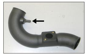
17. Install the provided 1/4npt fitting into the intake tube as shown.
