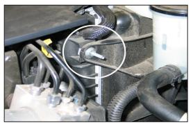
13. Remove the fan shroud mounting bolt shown.
