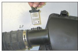
19. Remove the two screws which secure the mass air sensor and then remove the mass air sensor from the stock air box.
