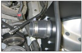
16. Install the provided step hose (084055) onto the filter adapter and secure with the provided hose clamp.
