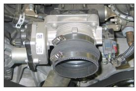
15. Install the provided hump hose (087121) onto the throttle body and secure with the provided hose clamp.
