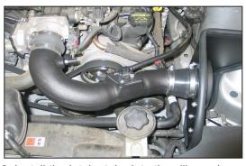
22. Install the intake tube into the silicone hose at the filter adapter and then into the hump hose at the throttle body and then secure with the provided hose clamps.
