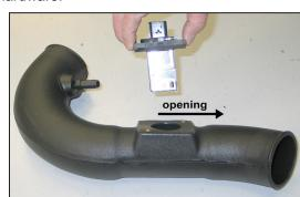
21. Install mass air sensor assembly into the intake tube and secure with the provided hardware.
