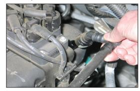
23. Remove the crank case vent tube assembly from the valve cover port.
