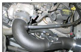
26. Reinstall the crank case vent hose assembly onto the valve cover and then connect the open end to the npt fitting installed into the intake tube. NOTE: It will be necessary to trim the silicone vent hose.
