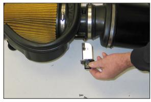
12. Remove the two screws securing the mass air sensor to the factory housing, then remove the mass air sensor as shown.
