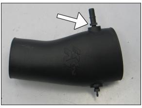
18. Install the quick disconnect fitting into the K&N® intake tube as shown.
