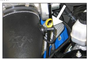
23. Connect the vent line to the 3/16" fitting installed into the K&N® intake tube.
