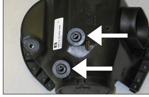
14. Remove the two factory mounting grommets shown from the airbox.
