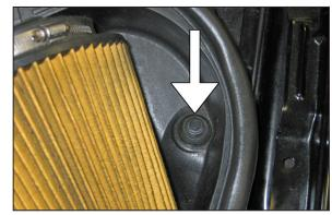
3. Remove the bolt that secures the airbox housing to the inner fender.
