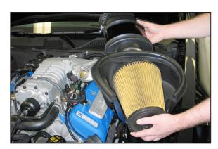
7. Disconnect the intake tube from the throttle body and then remove the complete intake system from the vehicle.
