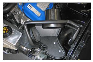
16. Install the heat shield assembly into the vehicle so the mounting bracket aligns with the factory airbox mounting location and the mounting grommets set into the mounting holes. Insert the fresh air duct into the heat shield.
