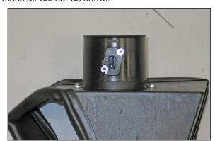
13. Install the mass air sensor into the K&N® mass air sensor housing and secure with provided hardware.
