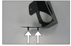
8. Install the heat shield mounting posts to the heat shield using the provided hardware as shown.
