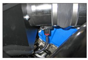
25. Reconnect the mass air sensor electrical connection.
