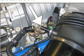
5. Rotate the locking ring and then disconnect the crankcase vent hose as shown.
