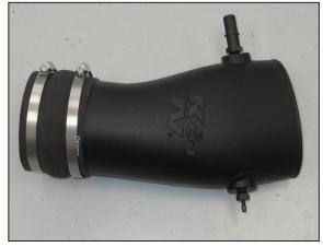
20. Install the provided silicone hose (08695) onto the K&N® intake tube, slide the hose all the way onto the K&N® intake tube; do not tighten at this time.
