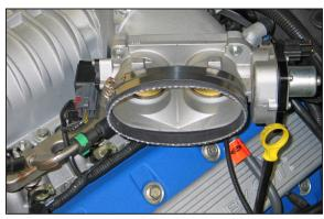
19. Install the provided silicone hose (08627) onto the throttle body and secure with the provided hose clamp.
