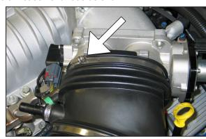
6. Loosen the hose clamp securing the stock intake tube to the throttle body.
