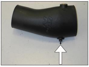
17. Install the provided 3/16" vacuum fitting into the  $K\&N^{\circ}$  intake tube as shown.
