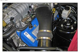
21. Install the K&N® intake tube into the silicone hose at the throttle body and align with the mass air sensor housing. Slide the silicone hose down the K&N® intake tube onto the mass air sensor housing. Align the tube for best fit and then secure with the provided hose clamps.
