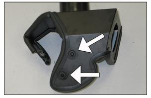
15. Install the factory mounting grommets to the two mounting posts installed on the K&N® heat shield assembly as shown.
