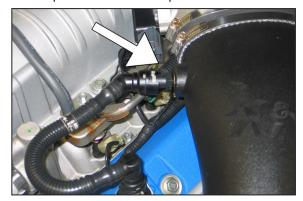
22. Connect the crankcase vent line to the quick disconnect fitting installed into the K&N® intake tube.
