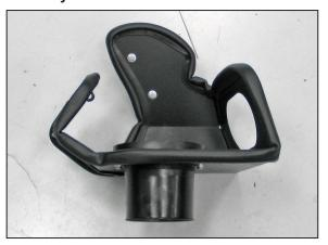
11. Install the mas air sensor into the heat shield, rotate the sensor 180° so the sensor boss is pointed downward, and then secure with the provided hardware.
