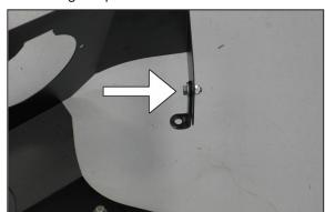
9. Install the heat shield mounting bracket (07158) onto the heat shield using the provided hardware.
