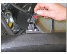
24. Connect the provided mass air sensor extension harness into the factory harness connection, and then connect the open end to the mass air senor electrical connector.
