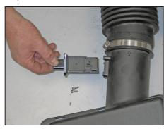
17. Remove the mass air sensor mounting bolts, then remove the mass air sensor from the factory air box.
