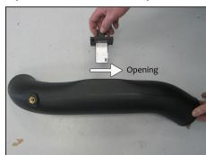
20. Install the mass air sensor assembly into the  $K\&N^{\otimes}$  intake tube as shown.
