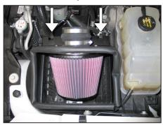
15. Install the completed heat shield / air filter assembly onto the lower air box and secure with the two factory air box retaining clips.
