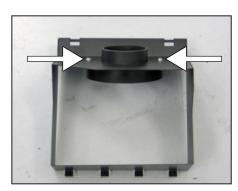
9. Install the K&N® filter adapter into the heat shield as shown and secure with the provided hardware.
