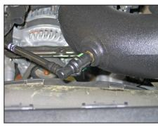
23. Rotate the crank case vent coupler so that it lines up with the fitting installed in the K&N<sup>®</sup> intake tube, then connect the coupler to the fitting.
