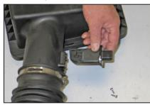
19. Remove the two screws securing the mass air sensor and then remove the mass air sensor from the stock intake tube as shown.
