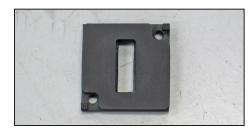
18. Install the provided gasket onto the mass air sensor adapter as shown.
