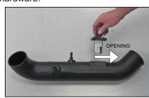
21. Install the mass air sensor assembly into the K&N<sup>®</sup> intake tube and secure with the provided hardware.
