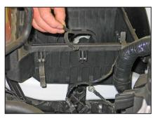
12. Remove the center airbox retaining clip.
