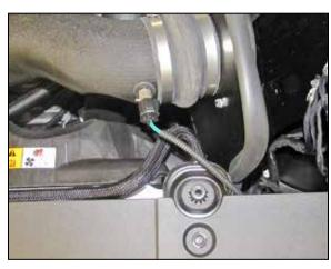
23. Connect the provided extension harness to the factory inlet air temperature sensor harness and then connect the other end to the inlet air temperature sensor as shown.
