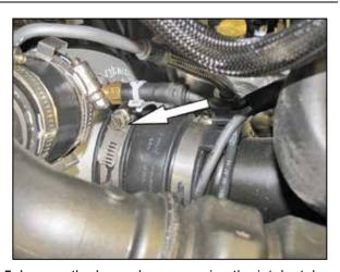
5. Loosen the hose clamp securing the intake tube to the Turbo.
