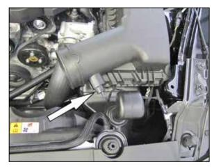
7. Disconnect the inlet air temperature sensor electrical connection.
