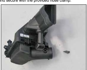
16. Remove the inlet air temperature sensor from the factory air filter housing.
