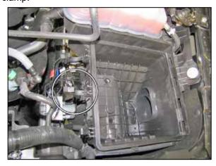
11. Remove the center upper air filter housing retaining clip as it will not be used.
