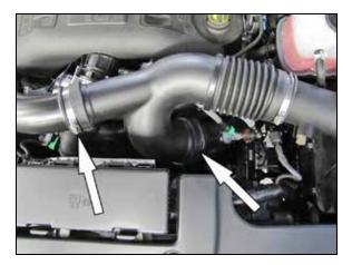
3. Loosen the three hose clamps that secure the factory intake tube and then remove the factory intake tube from the vehicle.
