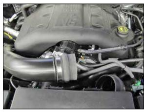
14. Install the provided hump coupler (087121) onto the passenger side turbo inlet tube and secure with the provided hose clamp.
