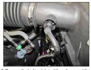
2. Depress the locking tab and then disconnect the inlet air temperature sensor electrical connection.
