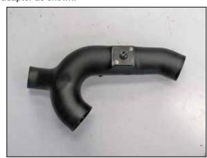
20. Install the inlet air temperature sensor assembly into the  $K\&N^{\circledcirc}$  intake tube and secure with the provided hardware.
