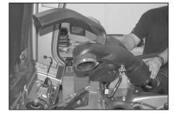
6. Detach the intake tube from the throttle body and mass air sensor then remove the intake assembly. **NOTE: On models equipped with a crank case vent tube, Disconnect the crank case vent tube from the port next to the valve cover and remove the tube with the intake tube assembly.**
