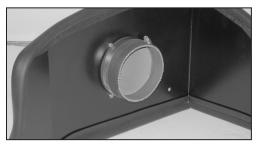
17. Install the silicone hose (08621) on the inside of heat shield with the provided hose clamps.
