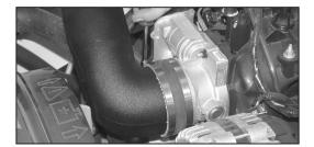
22. Align the intake tube with the throttle body then tighten the hose clamps.
