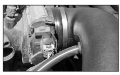
22d. Reinstall the K&N<sup>®</sup> intake tube and connect the provided crank case vent hose the hose mender and valve cover port. **NOTE: Some trimming of the hose will be necessary.**
