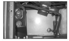
19. Secure the brackets to the heat shield with the provided hardware. Do not tighten completely.
