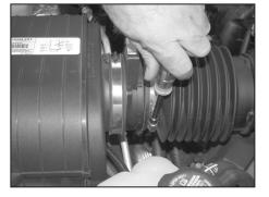
5. Loosen the hose clamp at the mass air sensor.
