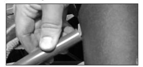
22a. On vehicles equipped with a crank case vent, install the provided crank case vent hose to the valve cover port and then align the hose to the K&N<sup>®</sup> intake tube in the straightest possible location. Mark this location on the intake tube and then remove the tube.
