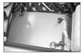
15. Install the 3 brackets onto the vehicle with the provided hardware as shown. Don't tighten completely at this time.
