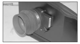
16. Install the silicone hump hose (08176) onto the mass air sensor with the provided hose clamps as shown.
