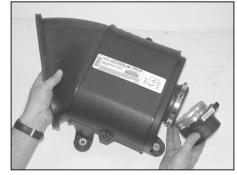
9. Loosen the hose clamp that retains the mass air sensor onto the air box then remove the mass air sensor from the air box.
