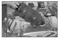
8. Remove the air box from vehicle as shown. NOTE: K&N Engineering, Inc., recommends that customers do not discard factory air intake. 11. Install the edge trim onto the heat shield. NOTE: Some trimming of the edge trim may be necessary.
