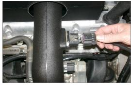
22. Reconnect the vehicles mass air sensor electrical connection.
