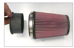
17. Install the filter adapter into the K&N $^{\odot}$  filter as shown.
