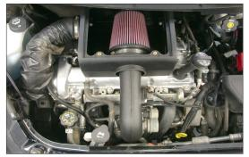
19. Install the K&N<sup>®</sup> intake tube through the opening in the air box and into the filter assembly. Then install the intake tube into the silicone hose at the throttle body and secure the filter and tube with the provided hose clamps.
