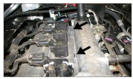
12. Install the two supplied 6mm studs into the valve cover as shown.
