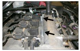
13. Thread and tighten the two coupling nuts onto the studs installed in step #12.
