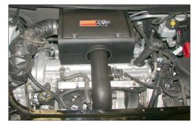
23. Reconnect the vehicle's negative battery cable. Double check to make sure everything is tight and properly positioned before starting the vehicle. 24. It will be necessary for all K&N<sup>®</sup> high flow intake systems to be checked periodically for realignment, clearance and tightening of all connections. Failure to follow the above instructions or proper maintenance may void warranty.
