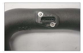
9. Secure the mass air sensor to the intake tube with the screws and spacers provided.
