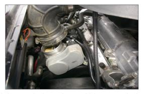
3. Loosen the hose clamp, which secures the intake tube to the throttle body, and then pull up on the intake tube/airbox assembly to dislodge it from the mounting grommets and disconnect the intake tube from the throttle body.
