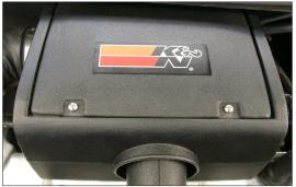
21. Install the K&N $^{\otimes}$  air box lid and secure with the provided hardware as shown.
