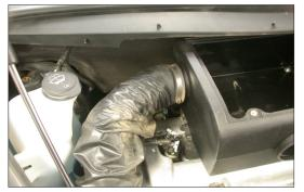
15. Install the fresh air supply hose onto the K&N<sup>®</sup> air box and secure with the factory hose clamp.
