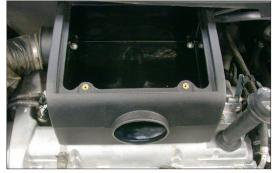
14. Install the K&N<sup>®</sup> air box onto the engine. Using the supplied hardware, secure the air box to the rear mounting bracket first and then to the coupling nuts installed in step #13.
