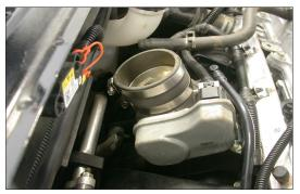
16. Install the silicone hose (08756) onto the throttle body and secure with the provided hose clamp.
