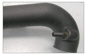
10. Install the supplied crank case vent fitting into the intake tube as shown.
