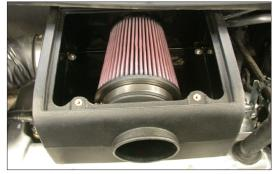
18. Place the filter assembly into the K&N $^{\mbox{\tiny \$}}$  air box as shown.
