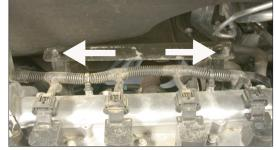
11. Remove the two stock air box mounting anchors shown from the mounting bracket.
