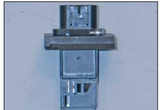
15. Install the mass air sensor into the K&N® mass air sensor adapter and secure with the provided hardware as shown.
