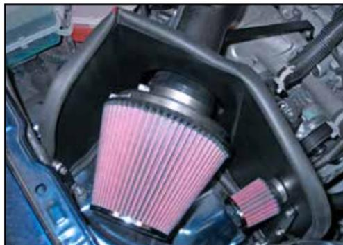
24. Install the air filter assembly onto the K&N® intake tube and secure with the provided hose clamp.
