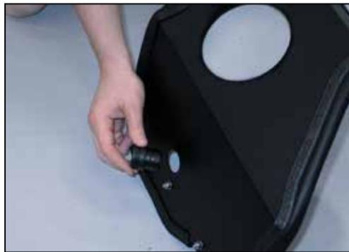
11c. Install the provided adapter into the small heat shield hole as shown.
