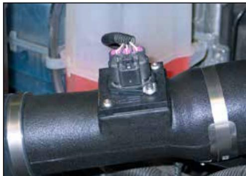
25. Re-connect the mass air sensor electrical connection.
