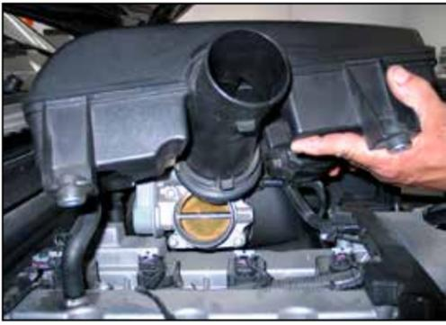
7. Remove the intake resonator from the vehicle as shown.
