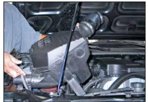
5. Lift the air box up, removing it from the vehicle.
