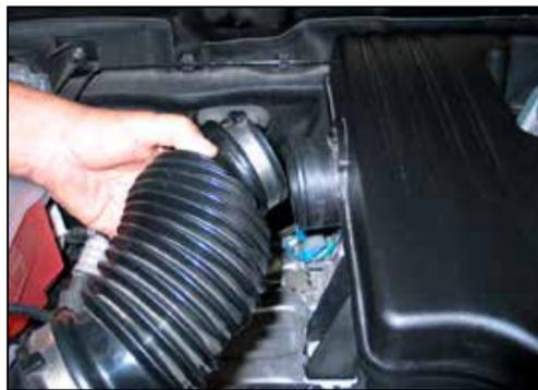
3. Loosen the hose clamp that secures the intake tube to the intake resonator. Disconnect the intake tube from the intake resonator as shown.
