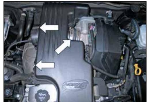
6. Loosen the two intake resonator mounting bolts and hose clamp at the throttle body.
