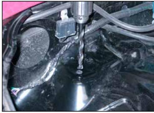
11a. On vehicles that are not equipped with the air box mounting stud and nut, drill out the existing hole in the inner fender with a drill and 1/2" bit.
