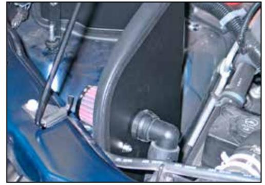
12a. On vehicles equipped with an air injection pump, secure the air injection pump hose to the adapter as shown.
