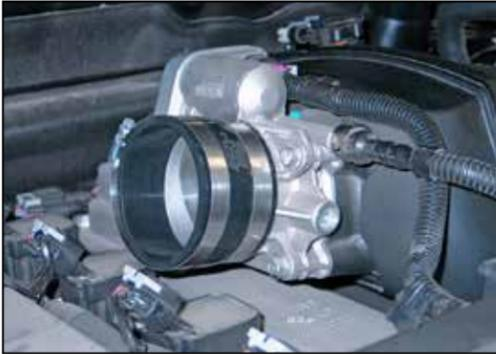
8. Install silicone hose (#08434) onto the throttle body and secure with the provided hose clamp as shown.
