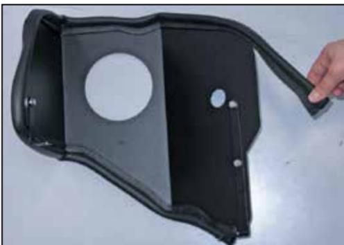
11. Install the edge trim onto the heat shield as shown.
