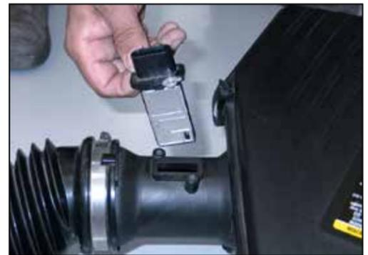
14. Remove the two mass air sensor mounting screws and remove the mass air sensor from the stock air box as shown.
