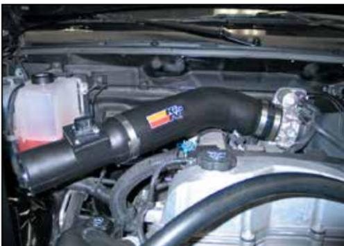
20. Install the K&N® intake tube into the silicone hose at the throttle body and align it with the mounting bracket installed in the previous step. Secure the intake tube with the provided hose clamps.
