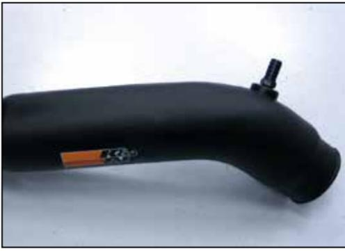
17. Install the provided 1/4" NPT fitting into the K&N® intake tube as shown.
