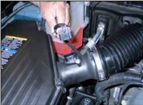
2. Depress the locking tab and disconnect the mass air sensor electrical connection.
