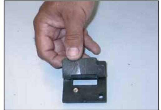
13. Install the provided gasket onto the K&N® mass air sensor adapter as shown.
