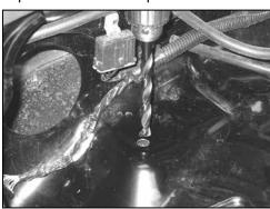
13a. On vehicles not equipped with the air box mounting stud and nut, drill out the existing hole in the inner fender with a  $\frac{1}{2}$ " drill.
