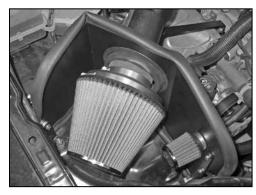
24. Install the air filter assembly onto the K&N® intake tube and secure with the provided hose clamp as shown.
