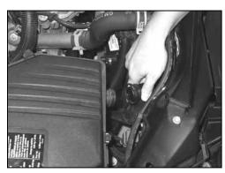
3. Depress the locking ring on the air pump fresh air inlet tube. Disconnect the fresh air inlet tube from the upper air box.
