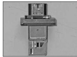
19. Install the mass air sensor into the K&N® mass air sensor adapter. Secure with the provided hardware.
