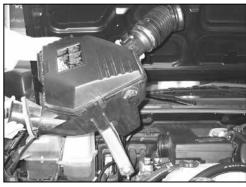
6. Lift the air box up, removing it from the vehicle as shown.
