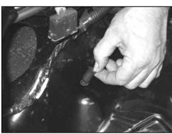
13b. Install the provided inserted nut into the hole drilled in step 13a.
