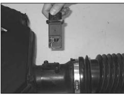
18. Remove the mass air sensor from the vehicle as shown.
