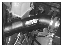
21. Install the K&N® intake tube into the silicone hose at the throttle body and align it with the tube mounting bracket installed in step 16. Secure with the provided hardware and hose clamp.
