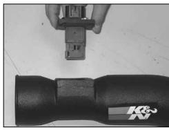
20. Install the mass air sensor assembly into the  $K\&N^{@}$  intake tube and secure it with the provided hardware.
