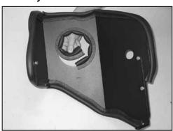
11. Install the small edge trim into the heat shield hole as shown.
