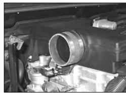
7. Install silicone hose (08630) onto the intake plenum and secure with the provided hose clamp as shown.
