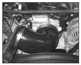
19. Install the 90° silicone hose (084053) onto the throttle body and secure with the provided hose clamp.
