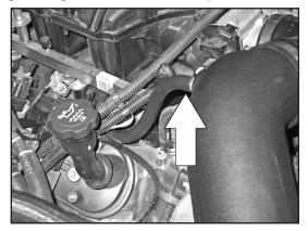
22. Install the supplied silicone hose onto the 1/4"npt fitting installed into the K&N<sup>®</sup> intake tube and then attach the open end onto the crank case vent port on the valve cover.
