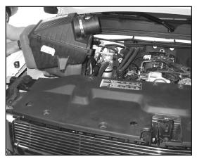
8. Firmly lift up the air box assembly to dislodge it from the mounting grommets. Then remove the air box assembly from the vehicle. **NOTE: K&N recommends that customers do not discard factory air intake.**
