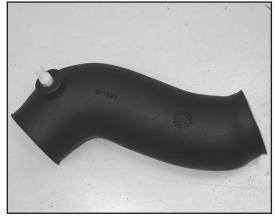
20. Install the  $\frac{1}{4}$ "npt fitting into the K&N<sup>®</sup> intake tube as shown.
