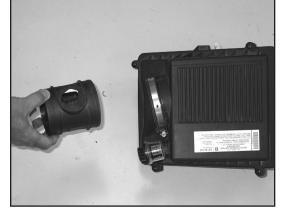
14. Loosen the hose clamp that secures the mass air sensor to the air box. Then remove the mass air sensor as shown.
