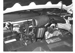
7. Unhook the stock intake tube from the mounting grommet and the upper radiator hose. Then remove the stock intake tube from the vehicle as shown.
