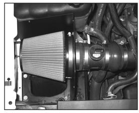
23. Install the K&N<sup>®</sup> Air Filter onto the filter adapter and secure with provided hose clamp. NOTE: Drycharger<sup>®</sup> air filter wrap; part # RF-1042DK is available to purchase separately. To learn more about Drycharger<sup>®</sup> filter wraps or look up color availability please visit
