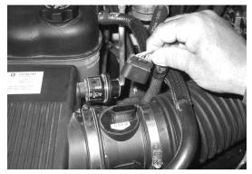
Disconnect the mass air sensor electrical connection.
