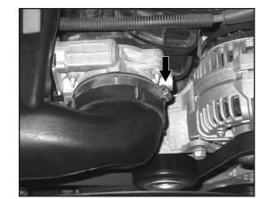
6. Loosen the hose clamp that secures the stock intake tube to the throttle body.
