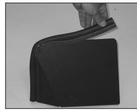
24. Install the edge trim onto the air box lid as shown.
