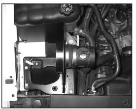
16. Install the heat shield assembly into the vehicle so that the inserted nuts fit into the air box mounting grommet holes. Then tighten the mounting bolts.
