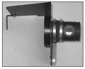
15. Install the mass air sensor onto the heat shield assembly and secure with the provided hose clamp.
