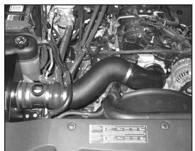
21. Install the K&N<sup>®</sup> intake tube into the throttle
