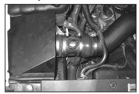
25. Install the air box lid and secure with the provided hardware.
