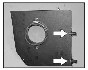
13. Install the two inserted nuts onto the heat shield as shown using the provided hardware. **NOTE: Do not completely tighten at this time.**
