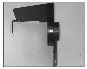
11. Using the provided hardware, install the filter adapter onto the heat shield as shown.
