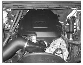
26. Install the engine cover back onto the engine.
