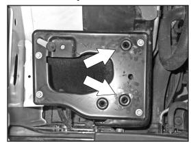
9. Remove the two pictured air box mounting grommets from the air box mounting plate.
