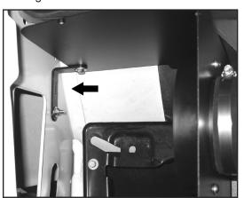
17. Secure the heat shield mounting bracket to the inner fender with the provided hardware.
