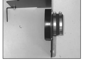
12. Install the silicone hose (08618) onto the filter adapter and secure with the provided hose clamp.
