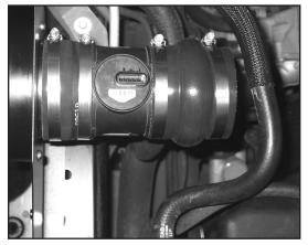
18. Install the silicone hump hose (084056) onto the mass air sensor and secure with the provided hose clamp.
