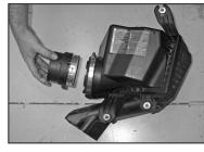
11. Loosen the hose clamp which secures the mass air sensor to the air box and then remove mass air sensor from the air box.
