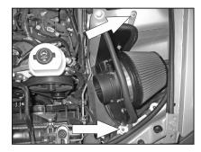
18. Install the heat shield assembly into the engine compartment and secure with the provided hardware.
