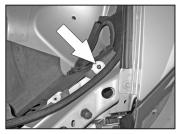
12. Secure the splash shield to the core support with the hardware provided.
