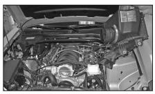
10. Remove the air box assembly from the vehicle. NOTE: K&N Engineering, Inc., recommends that customers do not discard factory air intake.
