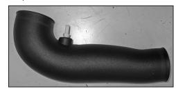
20. Install the crank case vent fitting into the K&N® intake tube as shown.
