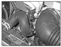
4. Release the crank case vent clip and then disconnect the crank case vent hose from the intake tube a shown.
