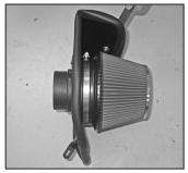
17. Install the K&N<sup>®</sup> air filter onto the filter adapter and secure with the provided hose clamp.
