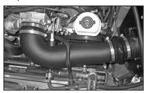
22. Install the K&N® intake tube onto the mass air sensor and then into the silicone hose on the throttle body. Secure the intake tube with the provided hose clamps.
