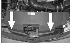
2. Release the two radiator cover retaining pins.
