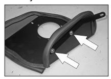
14. Install the heat shield mounting bracket (010126) onto the heat shield as shown using the provided hardware.
