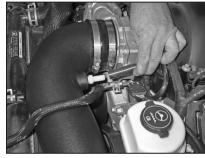
23. Install the provided crank case vent hose onto the valve cover and then connect the open end to the vent fitting on the K&N® intake tube.
