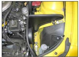
14. Install the heat shield assembly into the vehicle so the inserted nut goes into the air box mounting grommet hole and the tab goes onto the air box mounting stud. Secure the heat shield with the provided hardware.
