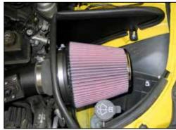
24. Install the K&N $^{\circ}$  air filter onto the filter adapter and secure with the provided hose clamp.
