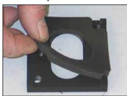
18. Peal the backing paper off and then install the provided gasket onto the K&N<sup>®</sup> mass air sensor adapter as shown.
