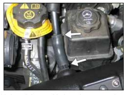
23. Install the provided crank case vent hose onto the factory crank case vent tube and then attach the open end to the vent fitting installed into the K&N® intake tube.
