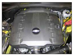
26. Reinstall the engine cover and secure with the oil fill cap.
