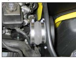
16. Install the provided silicone hump hose (08699) onto the filter adapter and secure with the provided hose clamp.
