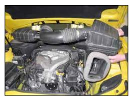
7. Remove the factory air box assembly from the vehicle.
