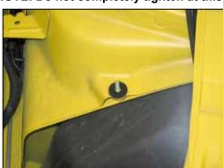
13. Install the provided rubber fender washer onto the outward air box mounting stud.
