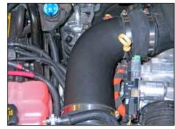
21. Install the K&N® intake tube into the silicone hose at the turbo inlet and then into the silicone hose at the mass air sensor. Adjust the tubes and mass air sensor housing for best fit and then secure with the provided hose clamps.
