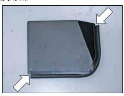
10. Install the 17.5" long section of edge trim onto the heat shield lid as shown.
