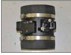
18. Install the two provided silicone hoses (08495) onto the K&N<sup>®</sup> mass air sensor housing as shown; secure with the provided hose clamps.
