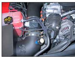
23. Connect the provided MAF extension harness into the factory wiring harness and then connect the open end to the MAF sensor. On models equipped with the second sensor, reconnect the electrical connection at this time also.
