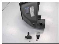
16. Remove the MAF sensors from the factory air box housing.
