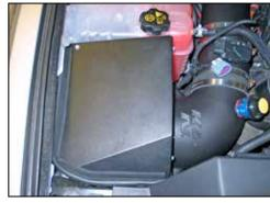
22. Install the heat shield lid onto the heat shield and secure with the provided hardware.
