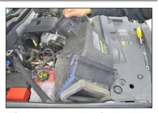
6. Lift up and remove the air box from the vehicle. NOTE: K&N Engineering, Inc., recommends that customers do not discard factory air intake.
