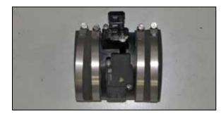
15. Install the two provided hoses (08495) onto the mass air housing and secure with the provided hose clamps.
