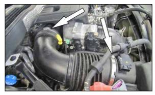
3. Loosen the hose clamps securing the factory intake hose to the air box and turbo inlet.
