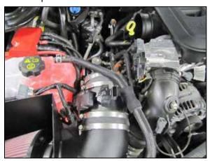
16. Install the Mass air assembly onto the K&N® intake tube as shown and secure with the provided
