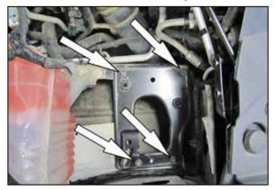
7. Remove the four bolts securing the air box mounting tray and then remove the tray from the vehicle
