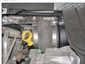
17. Install the provided hump hose (08633) onto the turbo inlet and secure with the provided hose
