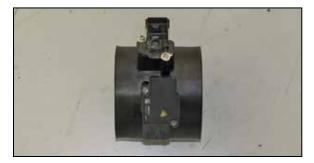
14. Install the sensors into the K&N® Mass air sensor housing and secure with the provided
