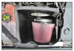
10. Set the K&N® air filter into the heat shield as shown.
