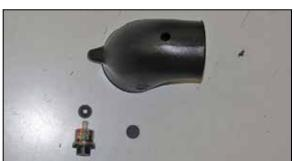
11. On vehicles equppied with a filter minder, remove the filter minder and grommet from the intake tube and install into the K&N intake tube. On vehicles that are not equipped with a filter minder, drill the hole in the K&N intake tube out to 7/8"ID and then install the provided plug into the tube.
