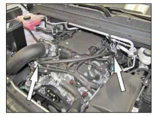
25. Install the crank case vent hose onto the fitting installed into the K&N® intake tube and then connect the hose mender into the fitting on the valve cover.
