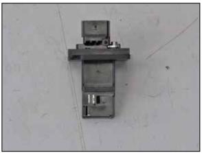
20. Install the factory mass air sensor into the K&N® adapter assemble and secure with the provided hardware.
