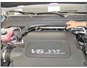
3. Disconnect the crank case vent hose from the intake plenum and then disconnect it from fitting on the valve cover.
