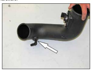
22. Install the provided 90° vent fitting into the K&N® intake tube as shown.
