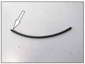
24. Install the hose mender into the provided crank case vent hose.
