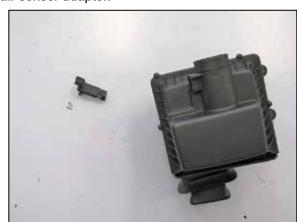
19. Remove the mass air sensor from the factory air filter housing.
