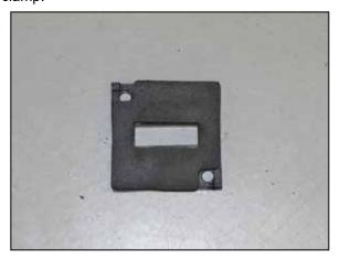
18. Install the provided gasket onto the K&N $^{\!0}$  mass air sensor adapter.
