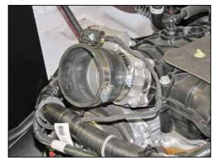
17. Install the provided step coupler (08724) onto the throttle body and secure with the provided hose clamp.
