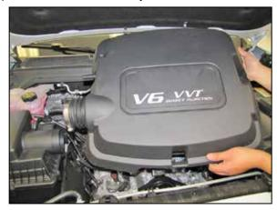
8. Lift up and remove the intake plenum from the engine.
