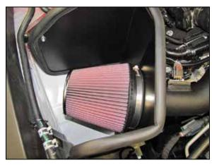
27. Install the K&N® air filter and secure with the provided hose clamp.
