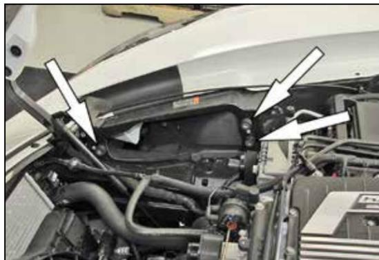
15. Install the three provided rubber mounted studs onto the air filter housing mounting locations as shown.
