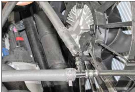
14. Cut 2" from the coolant hose and reinstall it onto the fitting and secure with the factory spring clamp.
