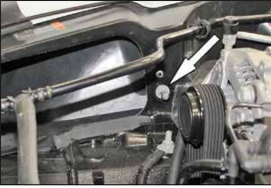
8. Remove the air filter housing mounting stud from the inner fender.
