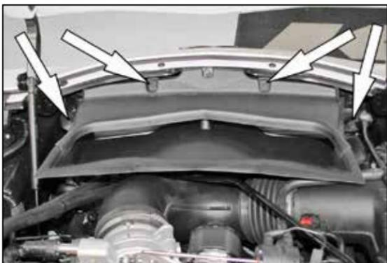
2. Remove the four bolts that secure the air extraction duct to the radiator and then remove the air extraction duct from the vehicle.
