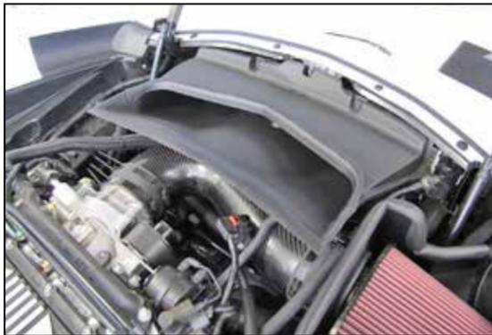
27. Reinstall the air extraction duct and secure with the provided hardware.
