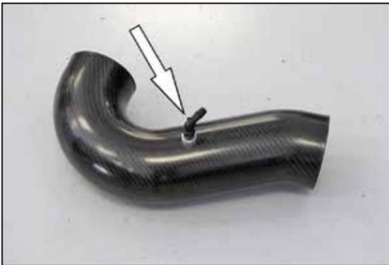
23. Install the provided 90° npt fitting into the K&N® intake tube as shown.
