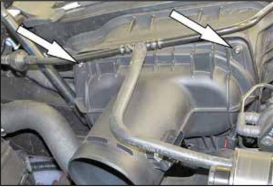
6. Loosen the two screws that secure the mass air sensor housing the air filter housing and then remove the housing and factory air filter.
