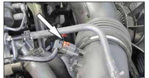
4. Release the red locking tab securing the mass air sensor electrical connection and then disconnect the mass air sensor electrical connection.
