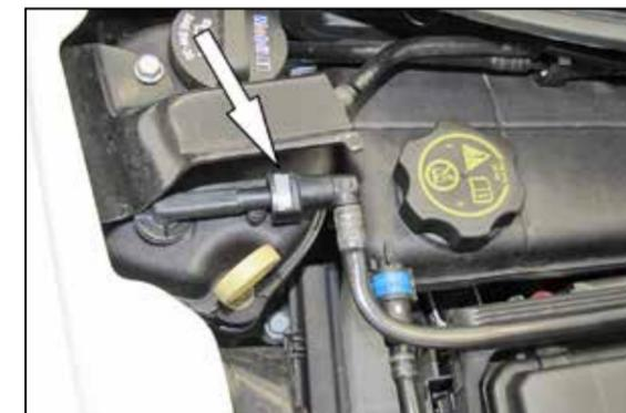
3. Release the grey locking tabs securing the crank case breather assembly to the factory intake tube and the oil tank. Then remove the crank case breather assembly from the vehicle.
