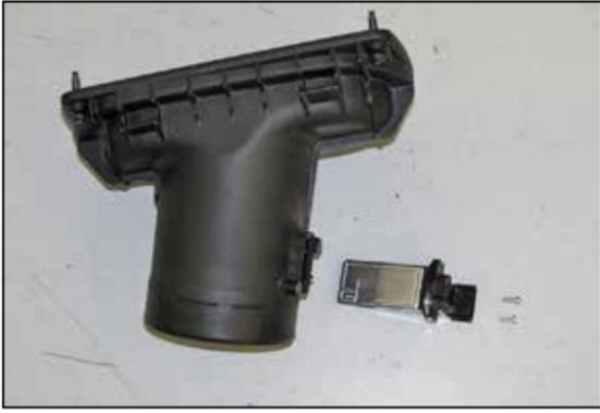
21. Remove the two screws that secure the mass air sensor into the housing and then remove the mass air sensor from the housing.
