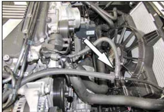
13. Release the spring clamp securing the coolant hose from the thermostat housing to the TEE fitting and then disconnect the hose from the TEE fitting.
