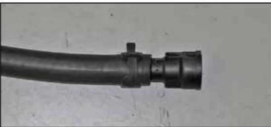
9. Assemble the coolant hose (08636), spring clamp and quick disconnect fitting as shown and then install the other spring clamp 1.5" from the open end of the hose as shown.
