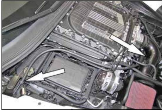
25. Install the provided crank case breather hose onto the fitting on the oil tank and then onto the fitting on the K&N® intake tube and secure with the provided spring clamps. Secure the hose as shown with the provided tie wraps.
