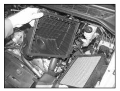
6. Release the two air box lid retainer clips that secure the air box lid to the air box, then remove the air box lid and air filter.
