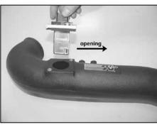
22. Install the mass air sensor assembly into the intake tube with the opening of the sensor pointing towards the air filter end of the tube as shown.
