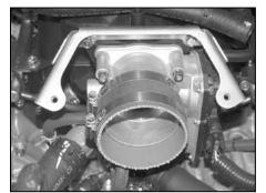
18. Install the provided silicone hose (08690) onto the throttle body with the provided hose clamps as shown.
