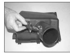
19. Remove the two screws that secure the mass air sensor to the air box lid, then remove the mass air sensor as shown.
