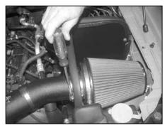
30. Install the K&N<sup>®</sup> air filter assembly onto the K&N<sup>®</sup> intake tube as shown; secure with the provided hose clamp.
