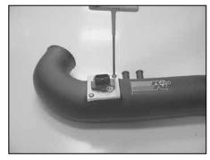
23. Secure the mass air sensor assembly onto the  $K\&N^{\circ}$  intake tube with the provided hardware.
