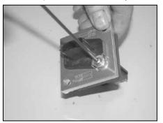
21. Insert the mass air sensor into the mass air sensor adapter and secure with the provided hardware.
