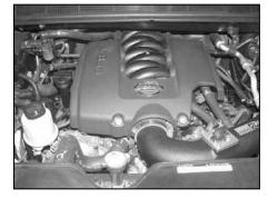
32. Re-install the throttle body cover as shown.
