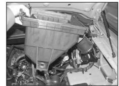
2. Remove the two bolts that secure the throttle body cover, then remove the throttle body cover.
