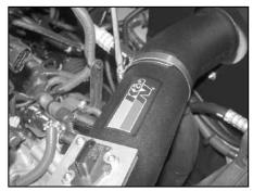
25. Secure the K&N<sup>®</sup> intake tube to the saddle bracket with the provided hose clamp. Also tighten the hose clamp at the throttle body.
