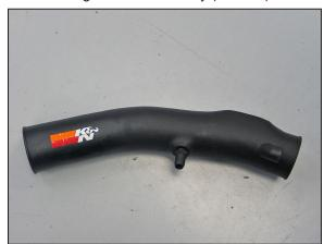
12. Install the  $\frac{1}{4}$ " NPT fitting into the K&N® intake tube as shown.
