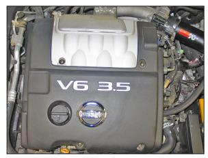
21. Re-install the engine cover and secure with the stock bolts.
