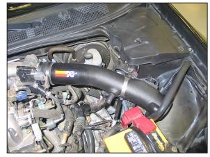
19. Install the K&N® intake tube assembly into the silicone hose at the throttle body and align with the saddle bracket installed in step #11. Secure the K&N® intake tube assembly with the provided hose clamps.
