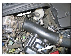
5. Loosen the two hose clamps that secure the stock intake tube to the throttle body and stock mass air sensor.
