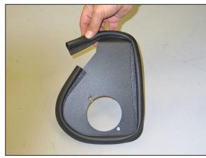
17. Install the provided edge trim onto the heat shield as shown.
