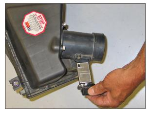
14. Remove the mass air sensor mounting screws. Then, remove the mass air sensor from the stock mass air sensor housing.
