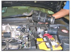
6. Remove the stock intake tube from the vehicle.
