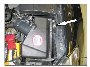
7. Remove the bolt that secures the airbox to the inner fender.
