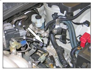
11a. On 2007 and later model vehicles, secure the tube mounting bracket assembly (070090).
