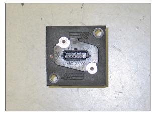
15. Install the mass air sensor into the K&N® mass air sensor adapter. Secure with the provided hardware.
