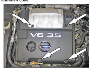
2. Remove the four bolts that retain the engine cover, then remove the engine cover from the engine.
