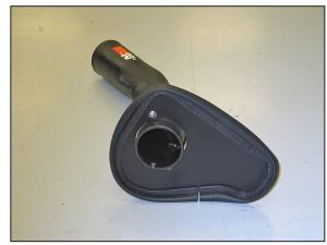
18. Secure the heat shield assembly to the K&N $^{\circ}$  intake tube with the provided hardware.
