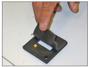
13. Install the provided gasket onto the K&N® mass air sensor adapter.
