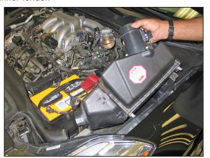
8. Lift the airbox up from the mounting grommets. Detach the airbox from the fresh air duct, then remove the airbox from the vehicle.
