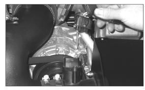
22. Pull the rubber wiring harness boot back from the mass air sensor electrical connector as shown. Rotate the connector 180 degrees and re-install the boot.
