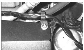
28. Re-attach the mass air sensor harness into the mass air sensor harness clip (mounted on heat shield) as shown.
