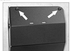
9. Install the two provided rubber bumpers onto the heat shield as shown.
