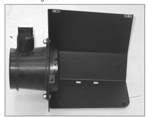
13. Install the mass air sensor housing into the heat shield and secure with the provided hardware as shown.
