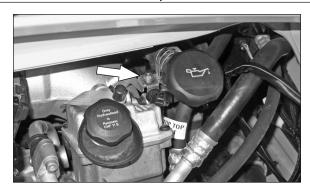
4. Remove the 10mm nut securing the harness clip, then remove the harness clip as shown. Re-install the 10mm nut and tighten. Set the harness clip aside for use in a later step.
