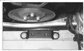
17. Install the heat shield bracket assembly into the grommet mounting holes as shown.
