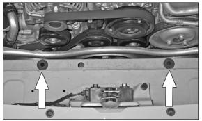
8. Remove the two air box mounting grommets as shown.
