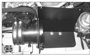
18. Install the heat shield assembly onto the heat shield bracket with the provided hardware as shown.
