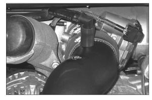
21. Re-connect the crank case vent line to the silicone hose installed in the previous step as shown.
