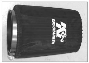
24. Install the provided  $K\&N^{\mbox{\scriptsize @}}$  Drycharger  $\mbox{\scriptsize @}$  onto the  $K\&N^{\mbox{\scriptsize @}}$  air filter as shown.
