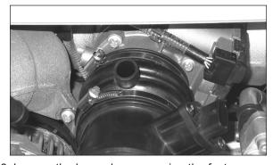
6. Loosen the hose clamp securing the factory intake tube to the throttle body as shown. Pull the factory intake tube from the throttle body.
