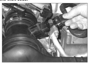
2. Depress the locking tab, then disconnect the mass air sensor electrical connection.
