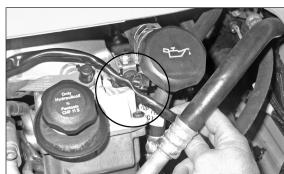
3. Release the mass air sensor clip (near the oil filler cap) as shown.
