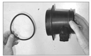
12. Remove the "O" ring seal from the mass air sensor housing as shown.
