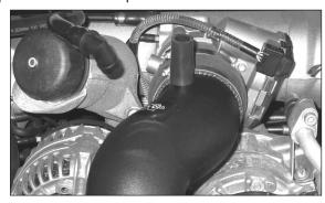
20. Install the provided silicone hose onto the  $K\&N^{\circledast}$  intake tube as shown.
