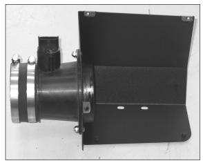
14. Install silicone hose (#08536) onto the mass air sensor housing and secure with the provided hardware as shown.
