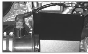
23. Route the mass air sensor harness and reconnect the mass air sensor electrical connector as shown.
