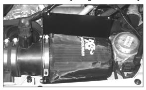
25. Install the K&N® air filter onto the K&N® intake tube and secure with the provided hose clamp as shown.
