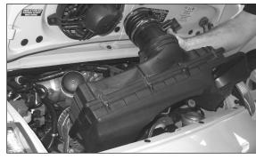
7. Pull up firmly, removing the factory air box and intake tube as shown.
