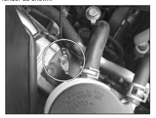
24. Using the bolt that was removed in the previous step, connect the ground strap to wheel well as shown.
