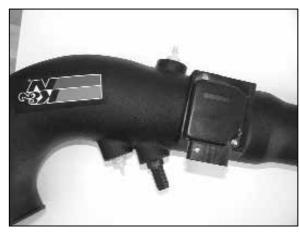
18. Assemble the vent fittings onto the K&N® intake tube as shown.
