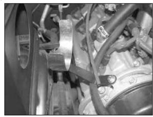
13. Install the saddle bracket assembly onto the threaded boss on the cam cover with the provided hardware as shown.
