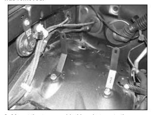
9. Mount the two provided brackets onto the vehicle with the provided hardware. NOTE: Bracket (07172) mounts closest to engine.
