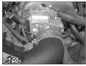
19. Install the K&N® intake tube onto the throttle body and align with the saddle bracket.
