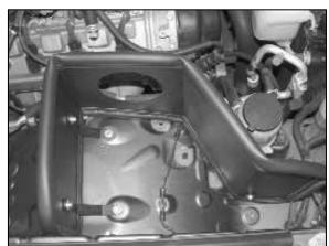
11. Install the heat shield onto the vehicle then secure to brackets with the provided hardware.
