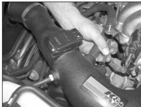
21. Install the provided silicone hose onto the  $K\&N^{\otimes}$  intake tube and re-connect the one existing vent line as shown.
