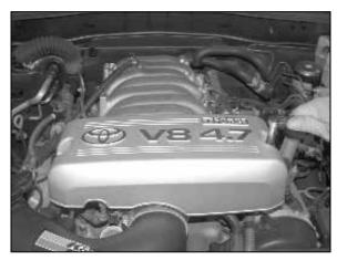
26. Re-install the throttle body cover as shown. Note: On Lexus GX470 models the Passenger side engine compartment panel will fit, light pressure will need to be applied down so the clips can be engaged. The cover can be left off if desired.
