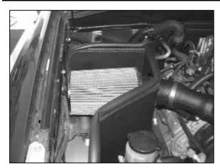
22. Install the K&N® air filter onto the intake tube as shown.
