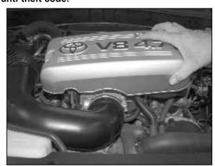
2. Loosen the two nuts that secure the throttle body cover then remove the throttle body cover. Note: The cover may be different. On Lexus GX470 models, the passenger side engine compartment cover panel will also need to be removed.
