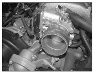
14. Install the provided silicone hose (08690) onto the throttle body with the provided hose clamp.
