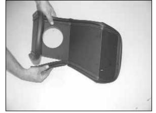
10. Install the edge trim onto the heat shield as shown. Trim if needed.
