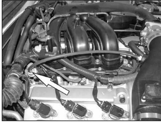
29. Remove the stock vacuum hose from fuel pressure regulator, then install provided silicone hose to fuel pressure regulator and then onto the K&N® intake tube.
