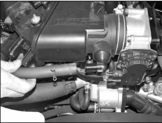
8. Remove crank case vent hose from air box as shown.
