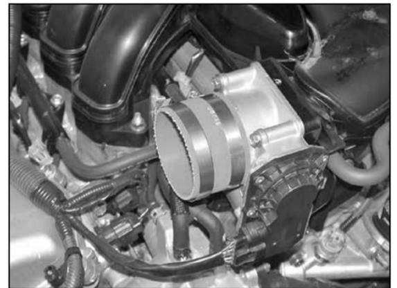
21. Install the provided silicone hose (08434) onto throttle body with the provided hose clamp as shown.
