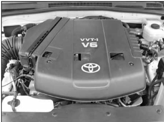
2. Loosen the two nuts that secure the engine cover, then remove the engine cover
