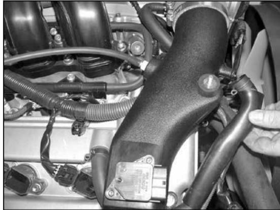
30. Fuel pressure regulator and then onto the K&N® intake tube. Install the original crank case vent hose onto the valve cover, then connect the crank case vent hose onto the K&N® intake tube.
