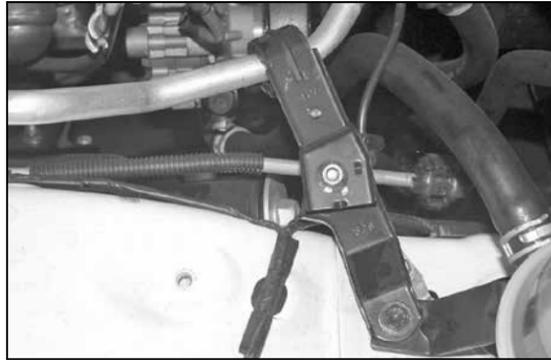
13. Rotate the A/C mounting bracket onto the power steering reservoir, then secure it using the bolt from the previous step. Tighten the A/C mounting nut.
