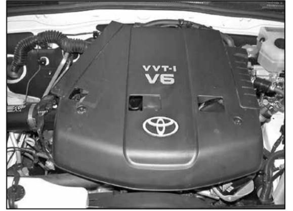
33. Re-install the engine cover using the original nuts removed in step #1.
