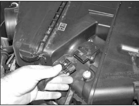
7. Disconnect the two mass air wire harness retaining clips from air box, then disconnect the mass air sensor electrical connection.
