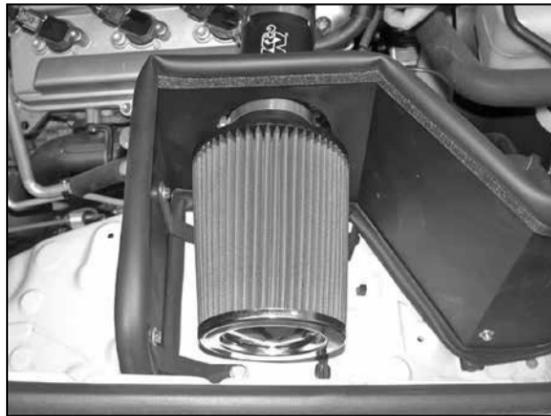
31. Install the K&N® Air filter onto the intake tube as shown.
