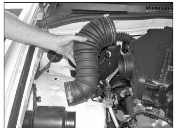
5. Remove intake tube from vehicle as shown.
