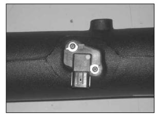
10. Install the mass air sensor into the K&N^ ${\rm e}$  intake tube and secure with the provided spacers and hardware as shown.
