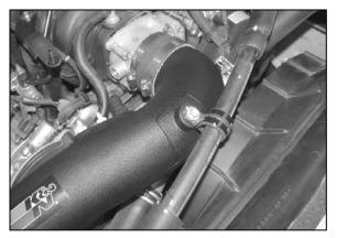
21. Attach the A/C hose to the intake tube with the bolt removed in step #4.
