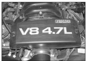
29. Reinstall the engine cover and secure with the nuts removed in step #3.
