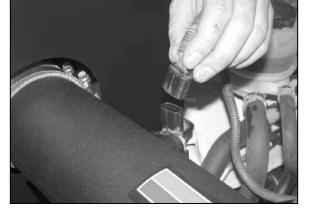
30. Reconnect the mass air sensor electrical connection as shown.
