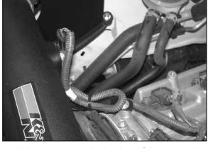
31. Using the provided wire tie, safely secure the excess mass air sensor wiring.
