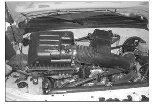
8. Remove the complete intake assembly from the vehicle as shown.
