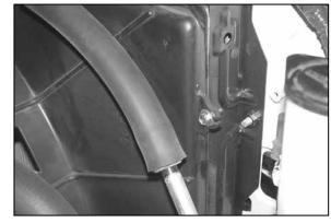
15. Remove the radiator fan shroud upper mounting bolt shown. **NOTE: This bolt will be reused.**
