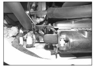
17. Secure the heat shield bracket to the radiator fan shroud with the bolt removed in step #15.
