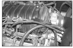
24. Install the provided fuel pressure regulator vent hose onto the fuel pressure regulator and then attach to the intake tube as shown.
