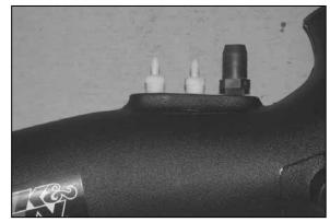
19. Install the provided npt fittings into the intake tube as shown.
