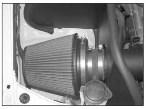
28. Install the air filter assembly onto the intake tube and secure with the provided hose clamp.
