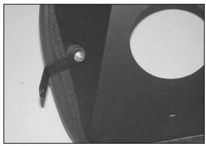
13. Install the provided bracket (070581) onto the rubber mounted stud installed in step #12. Do not tighten completely at this time.
