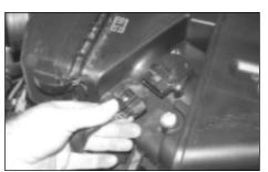
6. Disconnect the two mass air wire harnesses retaining clips from air box, then disconnect the mass air sensor electrical connection.
