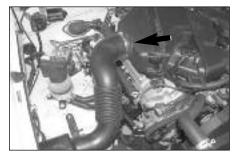
3. Loosen the intake tube hose clamp at the air filter assembly.
