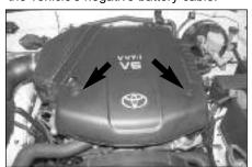
2. Loosen the two nuts that secure the engine cover, and then remove the engine cover from the engine.
