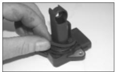
19. Apply the gasket to the mass air sensor, sticky side down as shown.
