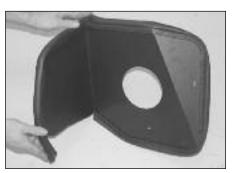
11. Install the provided edge trim onto the K&N intake tube as shown.
