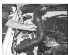
5. Remove the intake tube from the vehicle.
