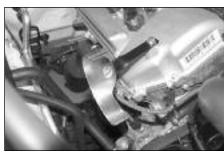
23. Install the tube mounting bracket onto the threaded boss on the valve cover with the provided hardware as shown.
