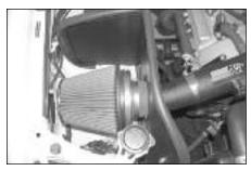
31. Install the Filtercharger assembly onto the K&N intake tube and secure with the provided hose clamp.
