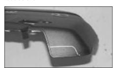
34. Using the provided template, mark the trim lines onto the engine cover and then cut with the appropriate tool.
