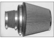
30. Install the silicone hose (08724) onto the Filtercharger assembly as shown and secure with the provided hose clamp.
