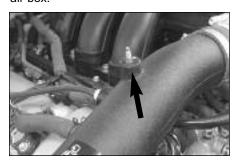
33. Install the engine cover mounting stud into the threaded stand off on the K&N intake tube as shown.
