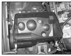
6. Remove the air box lid and filter to gain access to the three bolts that retain the air box to vehicle.
