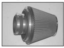
22. Install the silicone hose (08630) onto the K&N $^{\circ}$  Air filter assembly and secure with the provided hose clamp.
