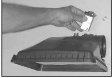
15. Remove the two screws that secure the mass air sensor to the air box lid, and then remove the mass air sensor as shown.
