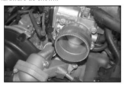
14. Install the provided silicone hose (08630) onto the throttle body with the provided hose clamp.
