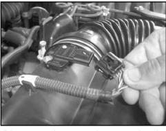
3. Disconnect the mass air sensor electrical connection, and then release the wiring from the air box.
