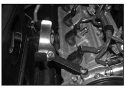
13. Install the saddle bracket assembly onto the threaded boss on the cam cover with the provided hardware as shown
