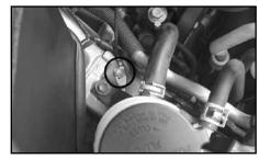
25. Using the bolt that was removed in the previous step, connect the ground strap to wheel well as shown.
