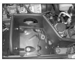
11. Install the heat shield onto the vehicle then secure to brackets with the provided hardware.
