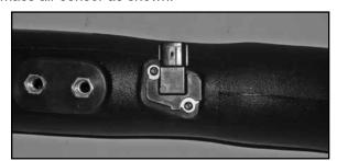
16. Secure the mass air sensor to the K&N<sup>®</sup> intake tube with the provided screws and spacers.
