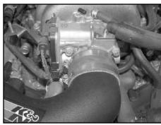
18. Install the K&N® intake tube onto the throttle body and align with the saddle bracket.
