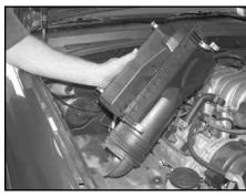
7. Remove the three bolts that retain the air box to vehicle, then remove the air box.
