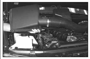
6. Release the four upper air box clam shell clamps, then remove the upper air box and intake tube assembly.
