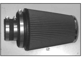
31. Install silicone hose (#08630) onto the air filter adapter and secure with the provided hose clamp.
