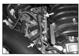
29. Install the provided fuel pressure hose onto the fuel pressure regulator, then connect the open end to the NPT fitting installed into the K&N® intake tube as shown.
