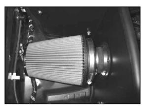
32. Install the K&N air filter assembly onto the K&N® intake tube and secure with the provided hose clamp as shown.
