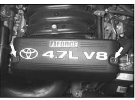
3. Remove the two factory nuts that retain the engine cover. Remove the engine cover.
