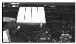
8. Lift the air box up, releasing it from the inner fender mounting grommet and fresh air duct. Remove the lower air box from the vehicle. Note: K&N recommends that customers do not discard factory air intake.
