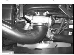
4. Loosen the hose clamp that secures the stock intake tube to the throttle body.
