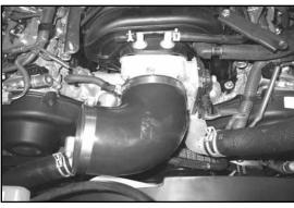
21. Install silicone hose (#084086) onto the throttle body and secure with the provided hose clamp.
