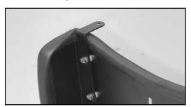
9. Install the small "L" bracket (#070742) onto the inner fender, behind the hood support. Secure with the provided hardware as shown.
