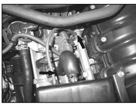
5. Disconnect the fuel pressure regulator hose from the fuel pressure regulator. Disconnect the crank case vent hose from the valve cover.
