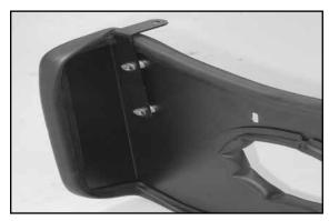
12. Install the long "L" bracket (#070902) onto the heat shield with the provided hardware as shown. Note: Place two of the provided spacers between the bracket and heat shield, one on each bolt.
