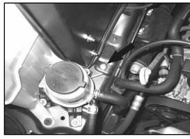
19. Secure the front heat shield bracket to the front air box location with the provided hardware.
