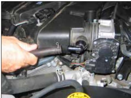
6. Disconnect the crank case vent hose from the air box as shown.
