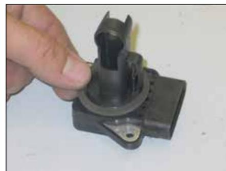
24. Install the mass air sensor gasket onto the mass air sensor as shown.
