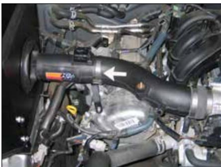
28. Install the K&N® Intake Tube assembly into the silicone hose at the throttle body and align with the tube mounting bracket assembly, then secure with the provided hose clamps.
