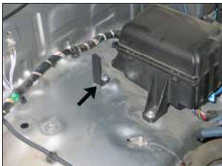
12. Install the "L" bracket (070089) onto the inner fender as shown.
