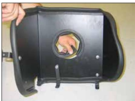
14. Install the provided edge trim inside the opening as shown.
