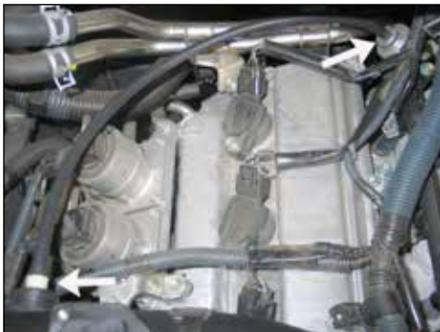
33. Install the provided vacuum hose onto the fuel pressure regulator and then attach the open end to the 1/4" npt fitting installed into the K&N® Intake Tube.
