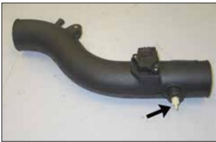
26. Install the 1/4" npt fitting into the K&N® Intake Tube as shown.
