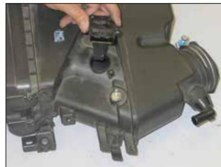
23. Remove the mass air sensor from the stock air box as shown.
