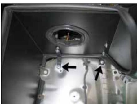
16. Set the heat shield assembly into position on the inner fender. Secure the lower mounting brackets to the inner fender using the factory nut and provided hardware.
