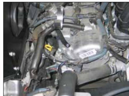
21. Install the tube mounting bracket assembly onto the valve cover using the provided hardware as shown.
