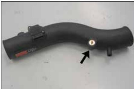
27. Install the provided rubber mounted stud onto the K&N® Intake Tube as shown.
