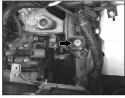
10. Remove the transmission mount bolt shown.
