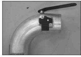
19. Install the mass air sensor into the  $K\&N^{\mbox{\scriptsize $\mathbb{R}$}}$  intake tube and secure with the provided hardware.
