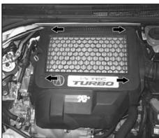
23. Reinstall the engine cover and secure with the factory quarter turn fasteners.
