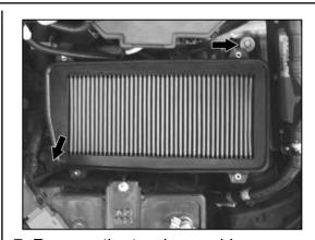
7. Remove the two lower airbox mounting bolts.
