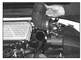
5. Remove the stock intake tube from the vehicle.
