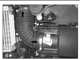
4. Loosen the two hose clamps that secure the intake tube to the airbox and turbo inlet tube.
