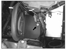
14. Install the heat shield assembly into the vehicle and secure to the engine mount using the bolt removed during step #10.
