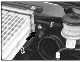
9. Remove the turbo inlet tube mounting bolt shown.
