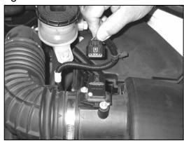
3. Disconnect the mass air sensor and unhook the wiring harness from the airbox and intake tube.
