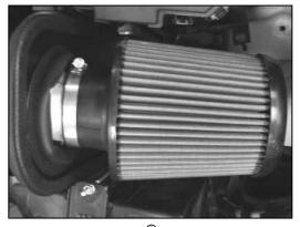
21. Install the K&N<sup>®</sup> air filter onto the intake tube and secure with the provided hose clamp.
