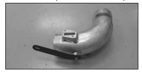
17. Install the supplied tube mounting bracket (070098) onto the K&N<sup>®</sup> intake tube using the provided hardware.
