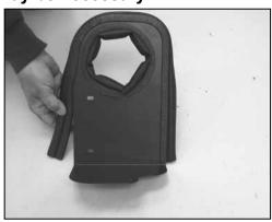
12. Install the long edge trim around the outside of the heat shield as shown. NOTE: Some trimming of the edge trim may be necessary.
