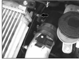
20. Install the K&N<sup>®</sup> intake tube into the silicone hose at the turbo inlet tube and align so the mounting bracket lines up with the turbo inlet mounting location. Secure the intake tube with the hose clamp and hardware provided.
