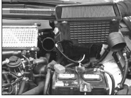
8. Lift and remove the lower airbox assembly.
