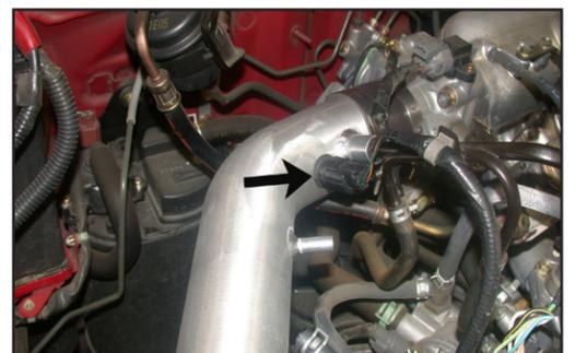
21. Insert the air temperature sensor into the grommet on the K&N® short ram tube as shown.
