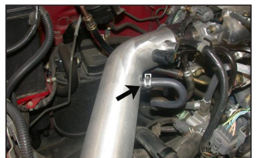
22. On vehicles with the FIAC valve connect the hose to the vent on the K&N® Typhoon® short ram tube as shown.
