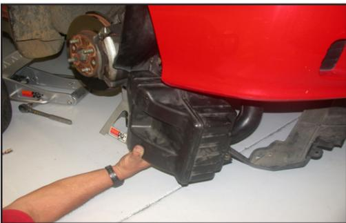
11. Remove the two bolts that secure the resonator to the inner fender, then, remove the resonator as shown.
