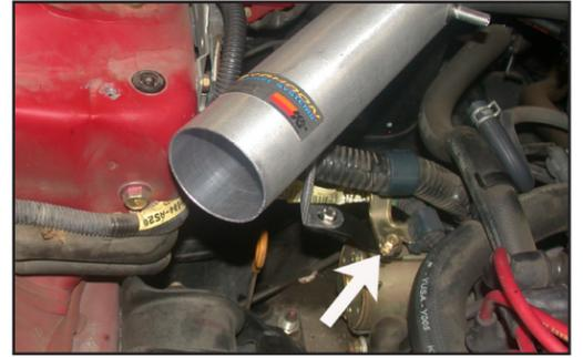
19. Slide the intake tube into the silicone hose on the throttle body, then, slide the "Z" bracket in between the starter bracket and the wire harness bracket, then, secure it using the stock bolt removed in step 16.
