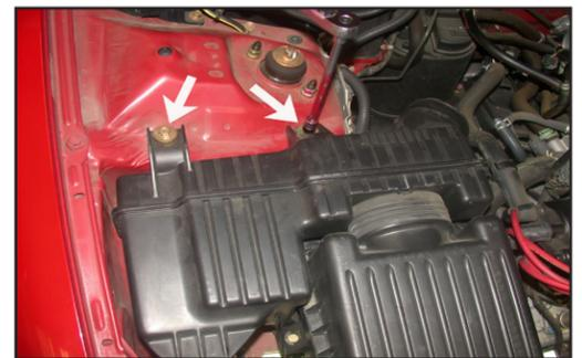
5. Loosen the two bolts on the air cleaner assembly as shown.
