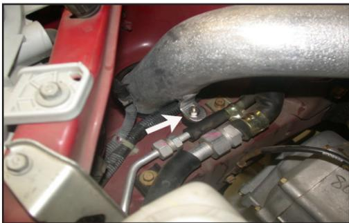
28. Secure the bracket to the rubber mounted stud using the provided hardware as shown, but do not tighten at this time.
