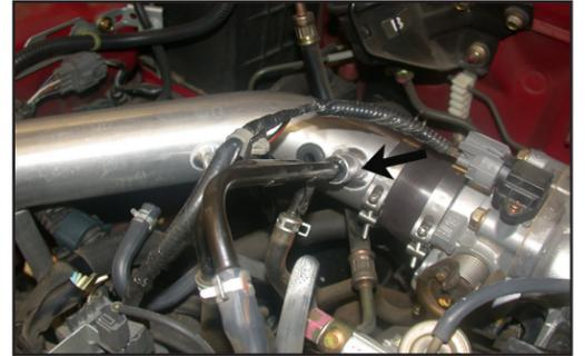
20. Insert the crankcase vent hard line into the vent on the K&N® Typhoon® short ram tube as shown.
