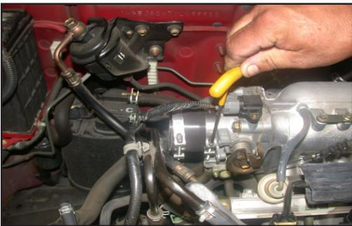
12. Install the silicone hose and hose clamps onto the throttle body and tighten as shown.
