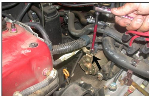
16. Remove the bolt that secures the wire harness bracket to the starter as shown.
