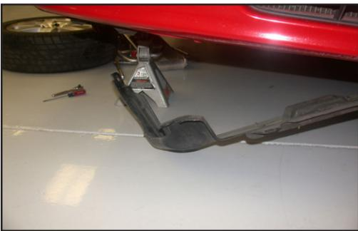
9. Remove the four plastic rivets/bolts, then, pull the lower splashguard down as shown.
