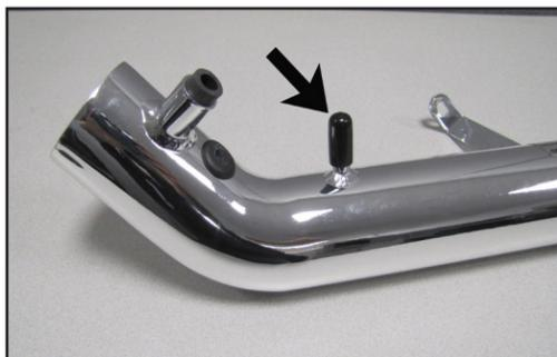
15. On models without the FIAC valve, plug the vent on the K&N® Typhoon® short ram tube with the provided cap plug.
