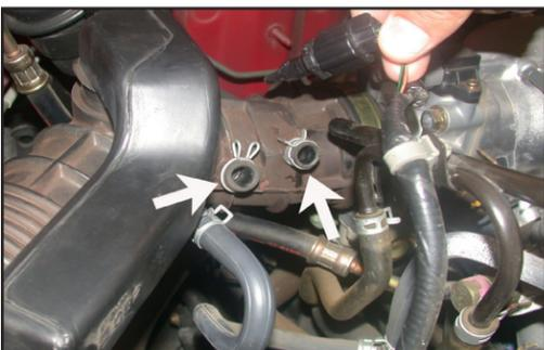
2. Disconnect the air temperature sensor and the crank case vent hard line from the stock intake tube.
