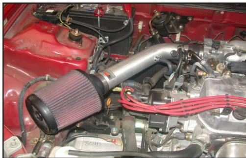
35. This K&N® Typhoon® kit has been designed to be used in two different configurations. In the case of inclement weather, the cold air tube can be removed and the air filter can be clamped onto the intake tube located in the engine compartment to avoid the possibility of ingesting water into the engine.
