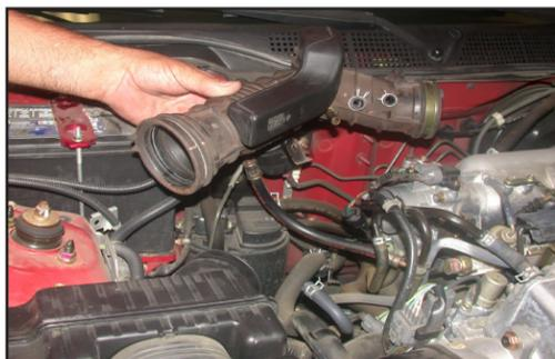
4. Loosen the hose clamp at the throttle body, then, remove the stock intake hose from the vehicle as shown.
