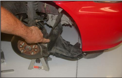
10. Remove the 2 plastic rivets and the 1 screw on the inner fender valance, then, pull the valance down as shown.
