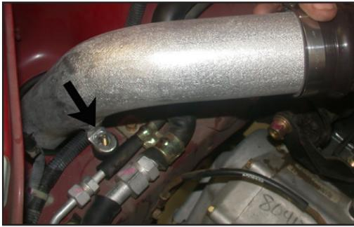
26. Install the cold air tube into the hole in the inner fender, then, line up the bracket with the rubber mounted stud as shown.
