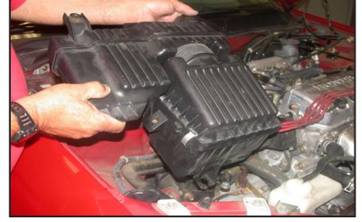
6. Pull firmly upwards to release the air cleaner from the lower grommet, then, remove the air cleaner assembly as shown.
