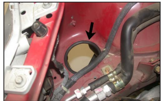
23. Install the provided edge trim onto the hole in the inner fender as shown.
