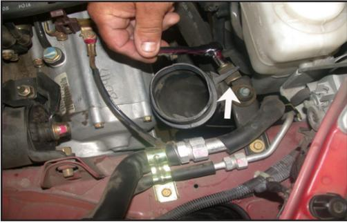
7. Remove the bolt that secures the air inlet tube to the inner fender as shown.
