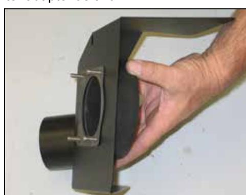
17. Install the air filter adapter into the heat shield as shown. Place the remaining gasket onto the exposed studs as shown.
