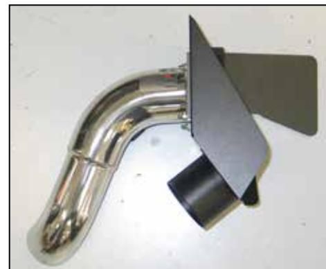
18. Install the K&N® intake tube onto the exposed studs and secure with the provided hardware.
