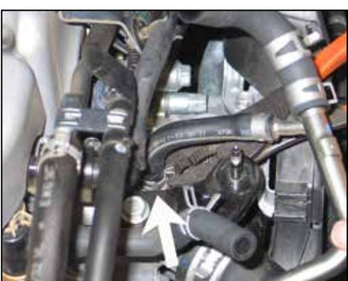
10. Ensure that the engine is not hot, then release the spring clamp that secures the coolant bypass hose to the intake manifold port. Disconnect the coolant bypass hose from the intake port.
