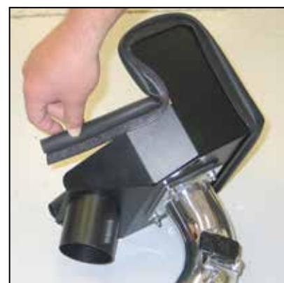
19. Install the provide edge trim onto the heat shield as shown.
