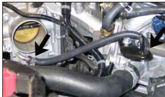
12. Install the provided bypass hose onto the throttle body and intake manifold ports. Secure with the provided hose clamps.
