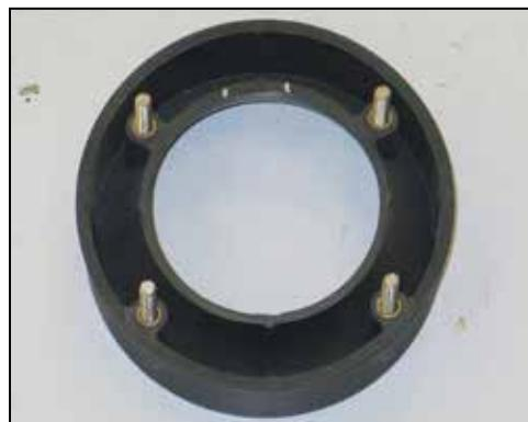
15. Install the four 6mm studs into the air filter adapter; threading them down until they bottom into the insert. tighten finger-tight.
