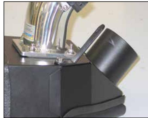
20. Install mounting bracket (#06507) onto the heat shield using the provided hardware as shown.
