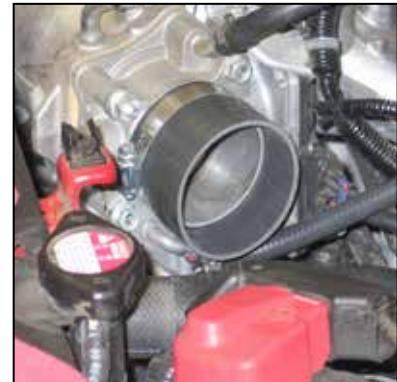
22. Install silicone hose (#08440) onto the throttle body and secure with the provided hose clamp.
