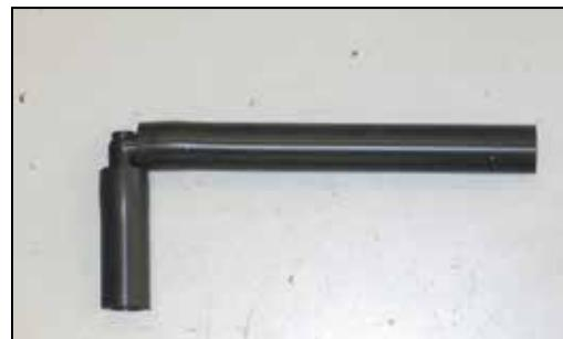
28. Assemble the crankcase vent hoses and provided 90° fitting as shown.
