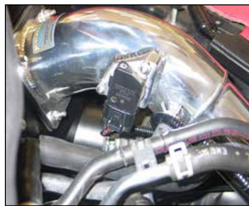
30. Re-connect the mass air sensor electrical connection.
