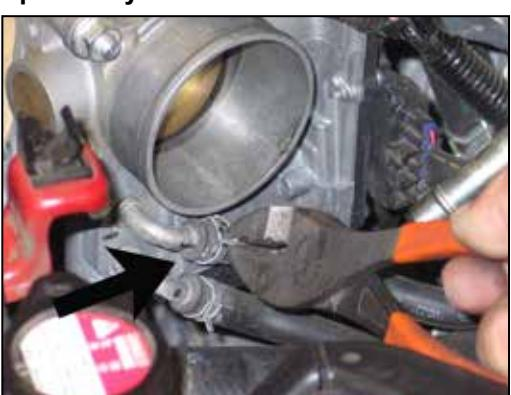
11. Release the spring clamp that secures the coolant bypass hose to the throttle body, then disconnect the coolant bypass hose from the throttle body. Remove the bypass/crank case vent hose assembly from the vehicle.
