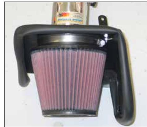
21. Install the K&N® air filter onto the air filter adapter and secure with the provided hose clamp.
