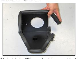
20. Install the 42" long edge trim around the heat shield.
