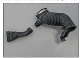
9. Separate the lower intake duct from the fresh air intake scoop.
