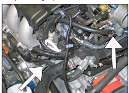
14. Remove the cap plugs and install the bypass hose onto the coolant fittings and secure with the provided hose clamps.
