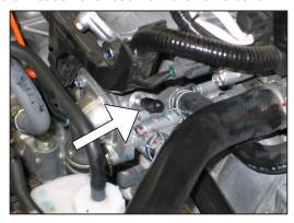
12. Release the spring clamp securing the coolant bypass hose to the thermostat housing. Remove the bypass hose from the thermostat housing fitting, quickly plugging the outlet with the remaining cap plug to prevent coolant loss. Remove the bypass/crankcase vent hose assembly from the vehicle.
