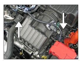
7. Remove the two bolts that secure the factory airbox.
