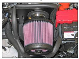
27. Install the K&N® air filter onto the intake tube and secure with the provided hose clamp.
