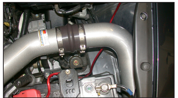
28. Slide the K&N® cold air tube through the hole in the inner fender and slide the tube into the silicone hump hose as shown. But do not tighten at this time.
