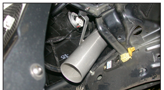
29. Line up the tube bracket with the rubber mounted stud and secure with the provided hardware as shown.
