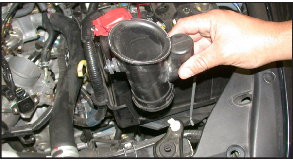
10. Remove the air inlet duct located directly in front of the battery.
