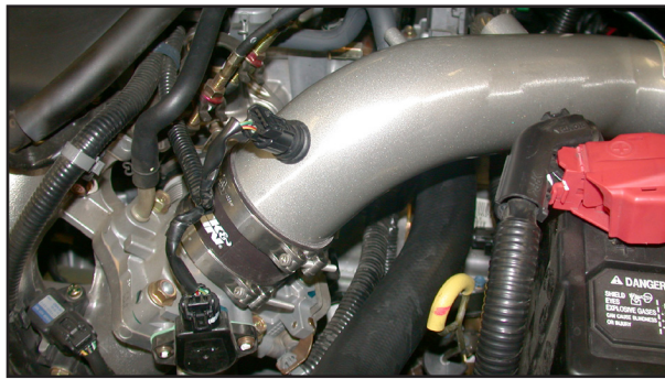
21. Install the air temperature sensor into the grommet as shown.
