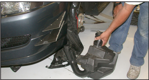
13. Remove the two bolts that secure the resonator to the inner fender, then, remove the resonator as shown.
