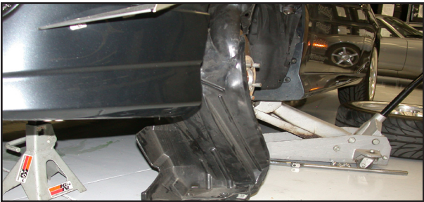
12. Remove the plastic rivets and screws that secure the inner fender valance, then, lower the inner fender valance down as shown.
