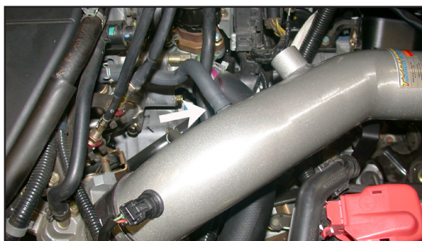
22. Reconnect the vent hose to the vent on the K&N® short ram tube as shown.
