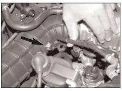
2. Disconnect the crankcase vent hose from the stock intake tube as shown.
