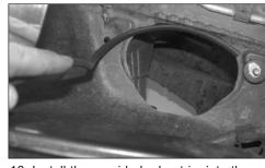
16. Install the provided edge trim into the hole in the inner fender as shown.
