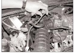
3. Remove the vacuum hose from the rubber clips on the stock intake tube as shown.
