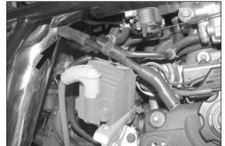
22. Slide the provided silicone hose onto the stock crank case vent hard line, then, secure the other end to the vent on the K&N® typhoon® short ram tube as shown.
