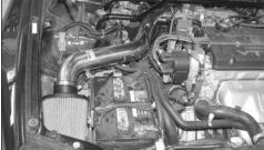
23. This kit is designed to be used in two different configurations. In the case of inclement weather, the cold air tube can be removed and the filter can be relocated onto the intake tube located in the engine compartment to avoid the possibility of ingesting water into the engine.
