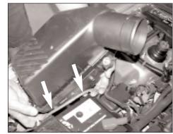
8.Pull upwards to remove the air cleaner assembly as shown.
