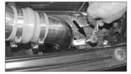
18. Using the provided hardware secure the bracket to the rubber mounted stud as shown.
