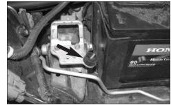
10. Install the rubber mounted stud into the stock bracket on the inner fender as shown.
