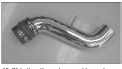
15. Slide the silicone hose and hose clamps onto the K&N® Typhoon® cold air tube as shown.
