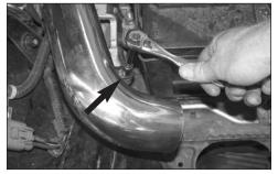
13. Using the provided hardware, secure the "Z" bracket to the rubber mounted stud as shown but do not tighten completely at this time.
