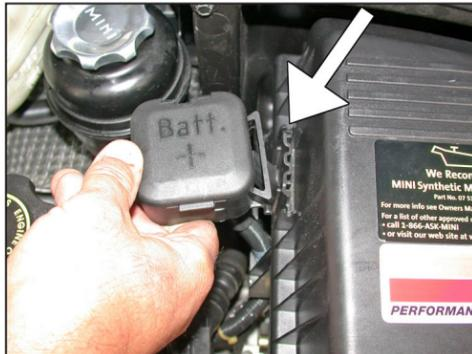
4. Pull upward to remove the battery terminal from the side of the air cleaner as shown.
