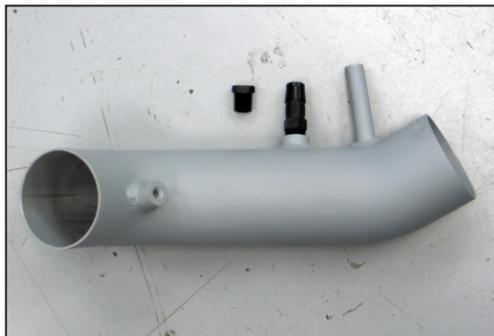
19a. On vehicles that come equipped with the additional vent line, install the provided vent fitting into the intake tube as shown. On all others install the provided plug.
