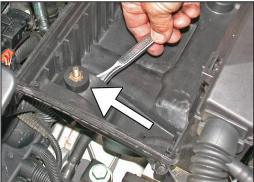
13. Secure the provided rubber mounted stud to the air inlet flange on the lower air cleaner assembly using the provided hardware as shown.
