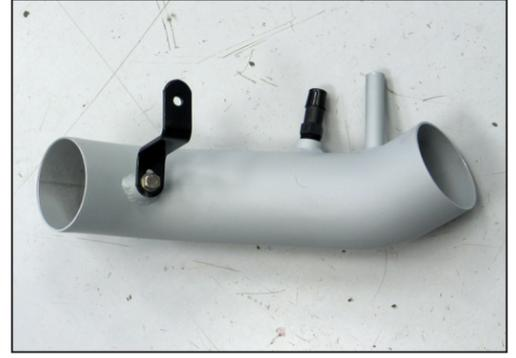
20. Secure the provided "Z" bracket onto the threaded boss on the K&N® intake tube using the provided hardware as shown.
