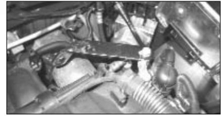
12. Mount the "L" bracket onto the engine using a washer and M6 bolt supplied as shown. (do not fully tighten at this moment)
