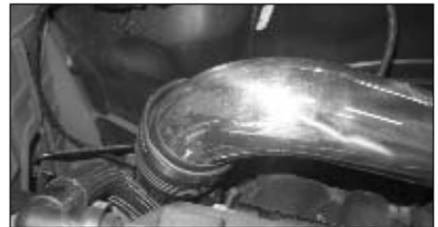
13. Fit the tube into the intake hose using the hose clamp supplied. (do not fully tighten at this moment.)
