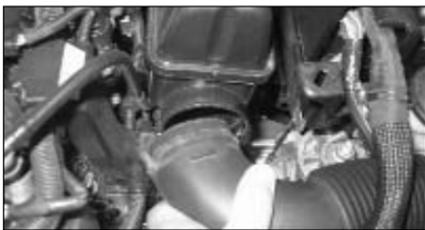
2. Remove the intake snorkel from the resonator box as shown.
