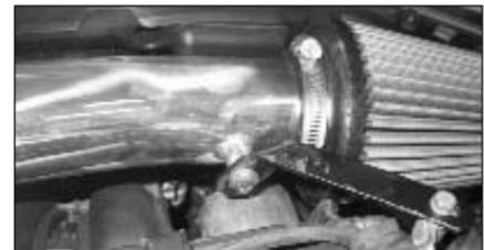
14. Fit the tube onto the "L" bracket using a washer, waved washer and M6 bolt supplied. Align the tube and tighten the hose clamp and M6 bolts.
