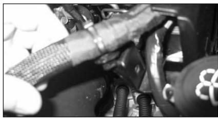
6. Carefully remove the wireloom from the ECU support bracket as shown.
