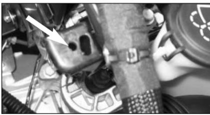
7. Carefully drill a 6.5mm hole in the ECU support bracket as shown.
