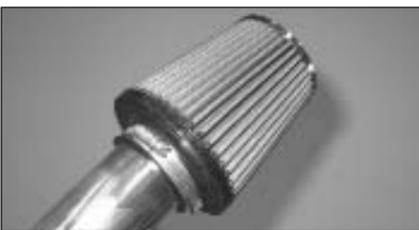
11. Clean the inside of the tube with water and a towel. Fit the filter to the tube using the hose clamp supplied.
