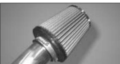
11. Clean the inside of the tube with water and a towel. Fit the filter to the tube using the hose clamp supplied.
