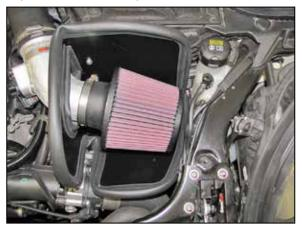
16. Install the K&N<sup>®</sup> air filter onto the intake tube and secure with the provided hose clamp. Adjust the tube and filter position for best fit. NOT LEGAL FOR SALE OR USE ON ANY POLLUTION CONTROLLED MOTOR VEHICLE IN CALIFORNIA OR STATES ADOPTING CALIFORNIA EMISSION PROCEDURES.
