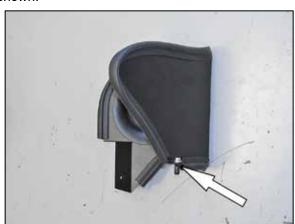
10. Install the provided heat shield mount onto the heat shield as shown.
