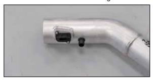
15. Install the mass air sensor into the K&N® intake tube and secure with the provided hardware.
