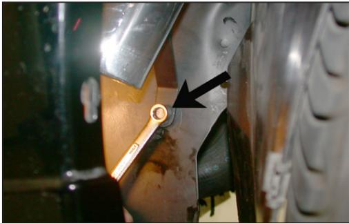
30. Line up the "Z" bracket with the hole on the inner fender and secure with the provided hardware as shown.
