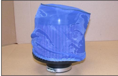
31. Slide the K&N® Drycharger® onto the K&N® air filter as shown.
