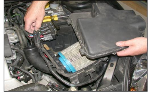
5. Loosen the five bolts that secure the air cleaner lid, then, remove the air cleaner lid as shown.
