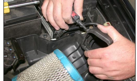
6. Remove the air temperature sensor from the air inlet duct as shown.
