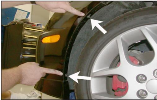
28. Remove the two screws that secure the inner wheel valance using a torx, size T25 as shown.
