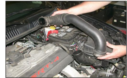
2. Loosen the hose clamp at the turbocharger inlet and at the air cleaner, then, remove the stock intake tube as shown.
