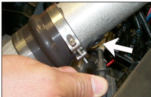
34. Install the air temperature sensor into the cold air tube as shown.
