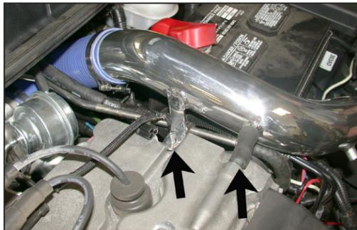
18. Slide the K&N® short ram tube into the silicone hose, then line up the tube bracket with the stud on the cam cover while sliding the silicone hose onto the vent on the cam cover as shown.
