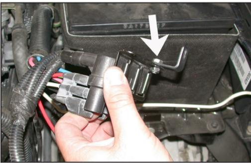
12. Secure the solenoid bracket to the provided "L" bracket using the provided hardware as shown.
