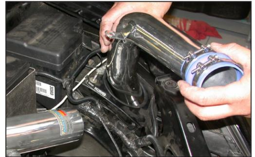
25. Slide the cold air tube into the hole in the inner fender as shown.
