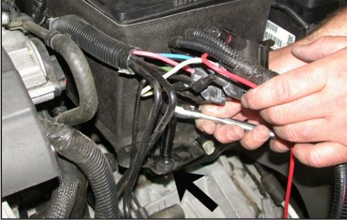
11. Remove the battery tray bolt as shown.
