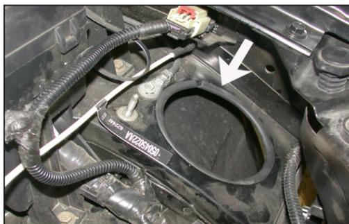
20. Install the provided edge trim onto the hole in the inner fender as shown.
