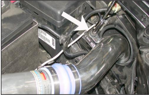
27. Secure the tube bracket to the stud using the nut removed in step 7 and the provided washer, but do not tighten at this time.
