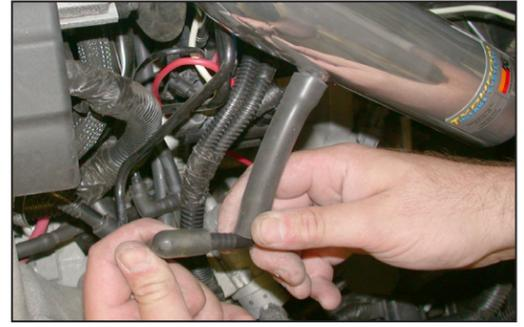
22. Slide the silicone hose onto the vent on the K&N® short ram tube, then connect the 90 degree vent to the stock vent as shown.
