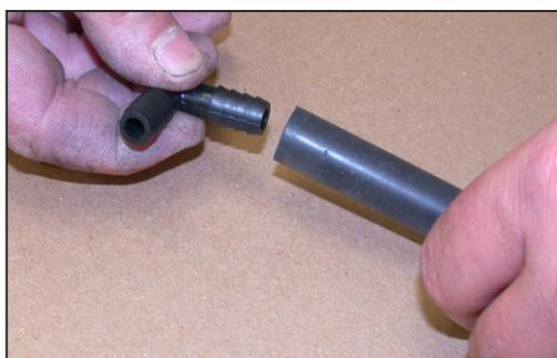
21. Install the 4-1/2" silicone onto the provided 90 degree vent as shown.
