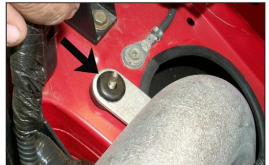
26. Line up the tube bracket with the original air cleaner mounting stud, then, slide the silicone hose onto the short ram tube as shown.
