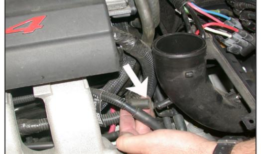
9. Disconnect the vent on the air cleaner tube as shown.
