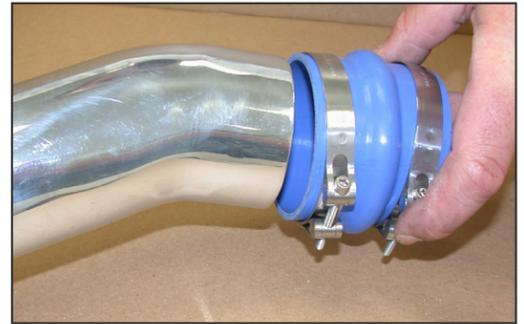
23. Slide the silicone hose and hose clamps onto the K&N® cold air tube as shown but do not tighten at this time.
