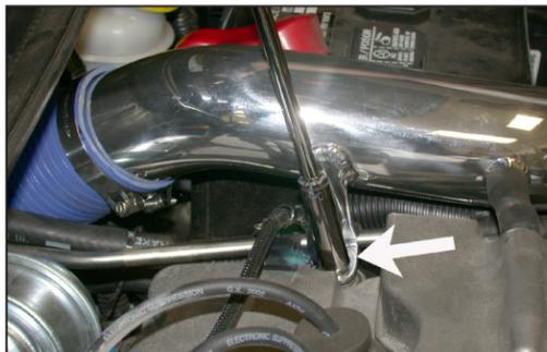
19. Secure the tube bracket to the cam cover using the nut removed in step 15 but do not tighten at this time.
