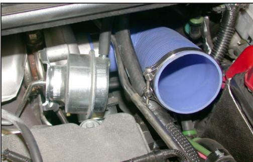
14. Install the silicone hose and hose clamps onto the turbo inlet but do not tighten at this time.
