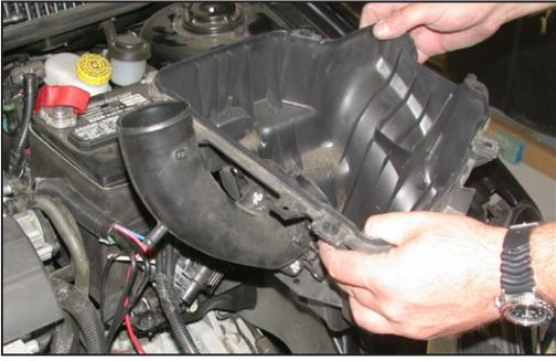
10. Pull firmly upwards to remove the lower air cleaner assembly as shown.
