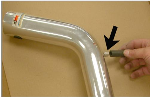
17. Cut a 2" length and a 4-1/2" length of silicone hose from the provided 10" length of silicone hose and install the 2" length hose onto the K&N® intake tube as shown.
