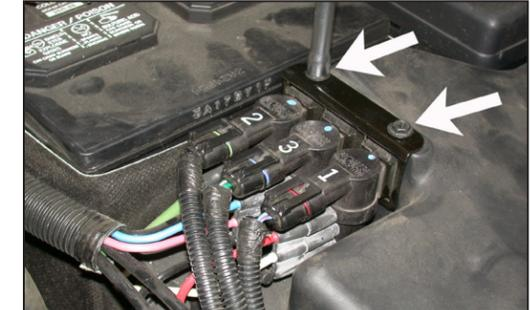
3. Loosen the two bolts that secure the solenoid bracket to the air cleaner assembly as shown.
