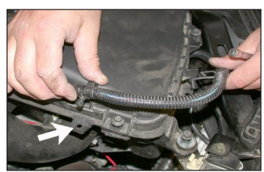
4. Unclip the wire harness from the air cleaner assembly as shown.
