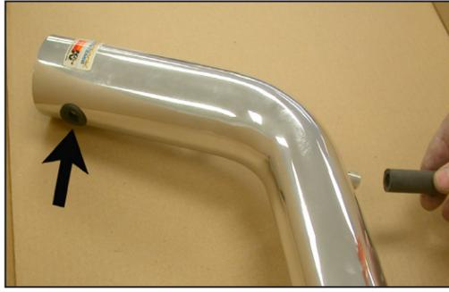
16. Install the provided grommet into the hole on the K&N® short ram tube.
