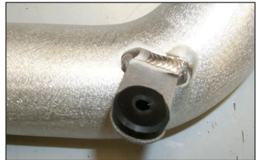
24. Insert the provided rubber grommet into the K&N® cold air tube bracket as shown.
