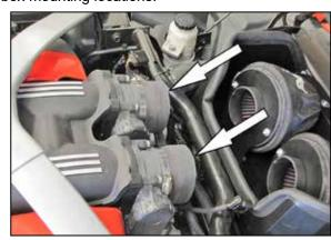
16. Install the two provided coupling hoses (08496) onto the throttle body and secure with the provided hose clamps.
