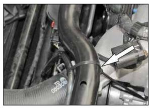
14. Secure the EVAP line to the frame cross member using the provided tie wrap.
