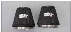
11. Install the provided "DRYCHARGER®" filter wraps onto the K&N® air filters as shown.
