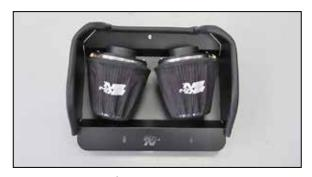
12. Install the K&N<sup>®</sup> air filter assemblies onto the filter adapters and secure with the provided hose clamps.
