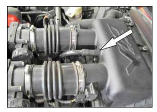
3. Disconnect the crank case vent hose from the factory air box.
