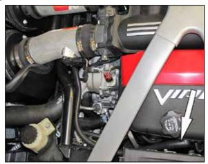
24. Connect the crank case vent hose to the factory elbow fitting with the union installed into the vent hose and then route the hose forward and install onto the 90° fitting installed into the K&N® intake tube.
