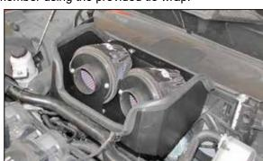
15. Install the heat shield assembly into the vehicle so that the inserted nut installs into the factory air box mounting grommet location. Secure the heat shield with the hardware provided to the factory air box mounting locations.
