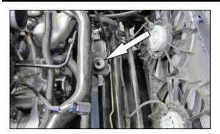
7. Remove the air box mounting grommet from the cross member.
