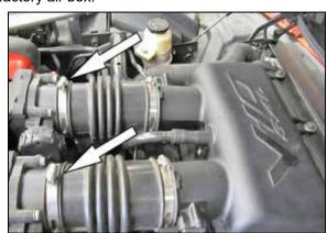
4. Loosen the two hose clamps which secure the factory intake tubes to the throttle bodies.
