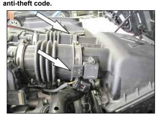
2. Unplug the two mass air sensor electrical connections.
