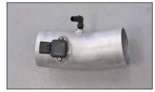
20. Install the provided 90° 1/4 npt vent fitting into the K&N® intake tube as shown.
