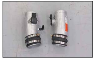
21. Install the provided hump hoses all the way onto the K&N® intake tubes as shown. Do not tighten at this time.
