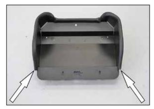
8. Install the provided edge trim onto the K&N® heat shield as shown.
