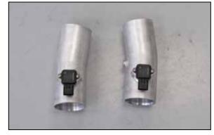
19. Install the mass air sensors into the K&N<sup>®</sup> intake tubes and secure with the provided hardware.
