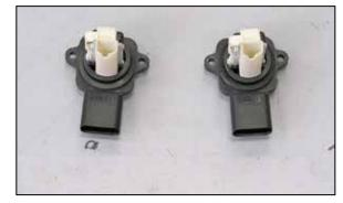
18. Remove the factory O-rings from the mass air sensor and then install the provided gaskets onto the sensors as shown.
