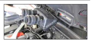
5. Remove the two thumb screws which secure the front of the factory air box to the core support, lift up the air box to unhook it from the mounting grommet. Disconnect the intake hoses from the throttle bodies and then remove the air box assembly from the vehicle.
