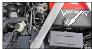
6. Unhook the crank case vent tube retaining clip from the frame cross member. Remove the crank case vent tube from the 90° fitting at the valve cover and then remove the tube from the vehicle. NOTE: On later model vehicles, due to the crank case vent being relocated it will be necessary to remove the decorative engine cover to access the connection.
