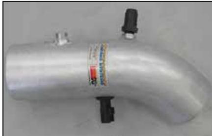
19. Install the inlet air temperature sensor into the grommet installed into the K&N® intake tube.
