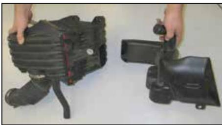
12. Disconnect the fresh air scoop from the airbox as shown.
