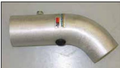
15. Install the provided grommet into the K&N® intake tube as shown.
