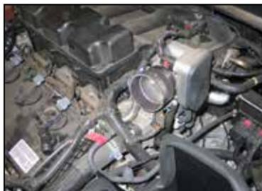
20. Install the provided silicone hose (084036) onto the throttle body and secure with the provided hose clamp.
