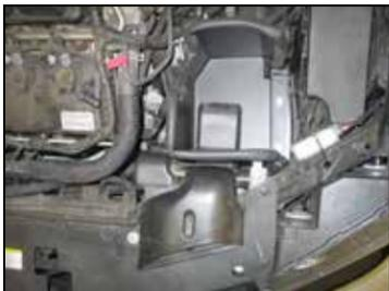
14. Install the heat shield assembly onto the frame rail. Secure the heat shield assembly to the factory airbox mounting locations with the factory bolt and hardware provided. Secure the fresh air intake scoop to the core support using the factory mounting pin.
