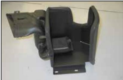
13. Install the fresh air scoop into the heat shield as shown.
