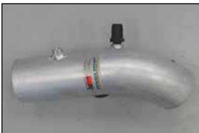
16. Install the provided NPT fitting into the K&N® intake tube as shown.
