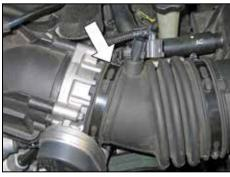
5. Loosen the hose clamp securing the intake tube to the throttle body.
